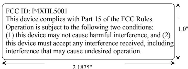
Specifications: Text is black in color and is left justified. Labels are printed in indelible ink on permanent adhesive backing and shall be affixed at a conspicuous location on the EUT.
