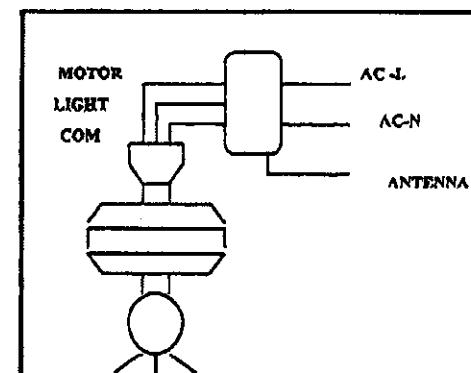
Figure 3 install receiver ceiling fan chart
