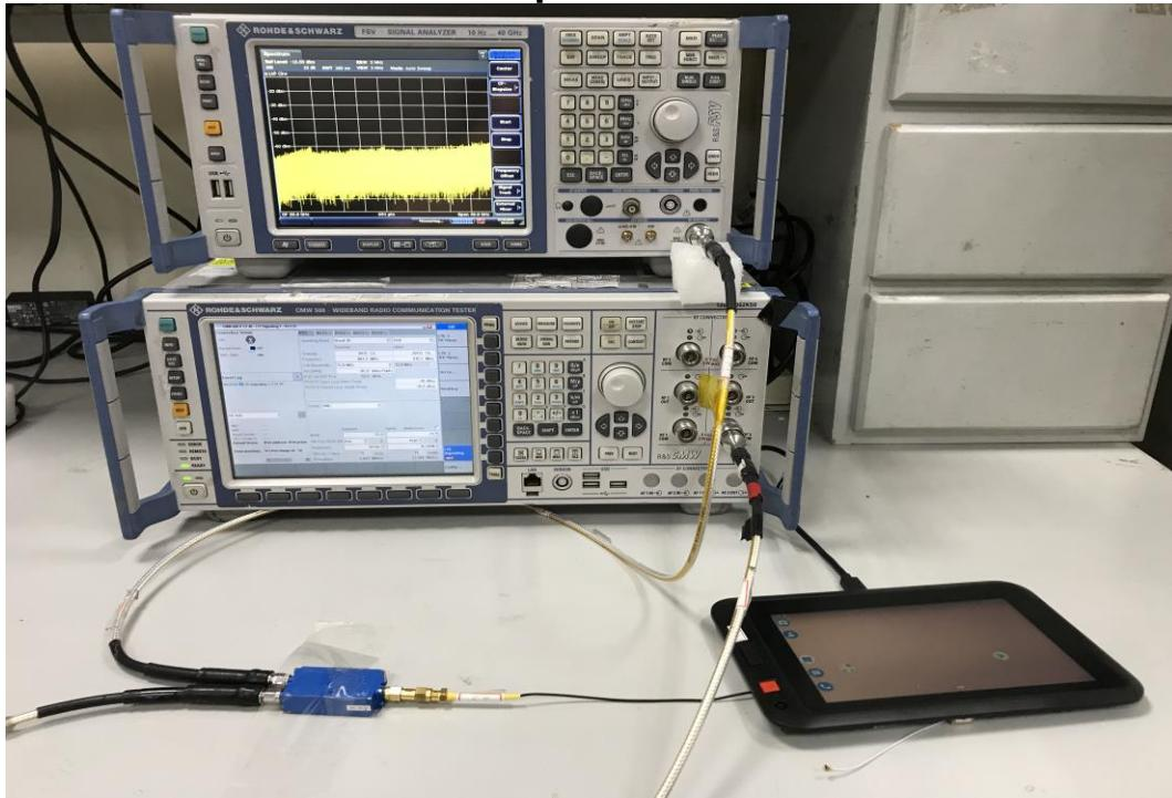
**Radiated Emission Set up Photos
