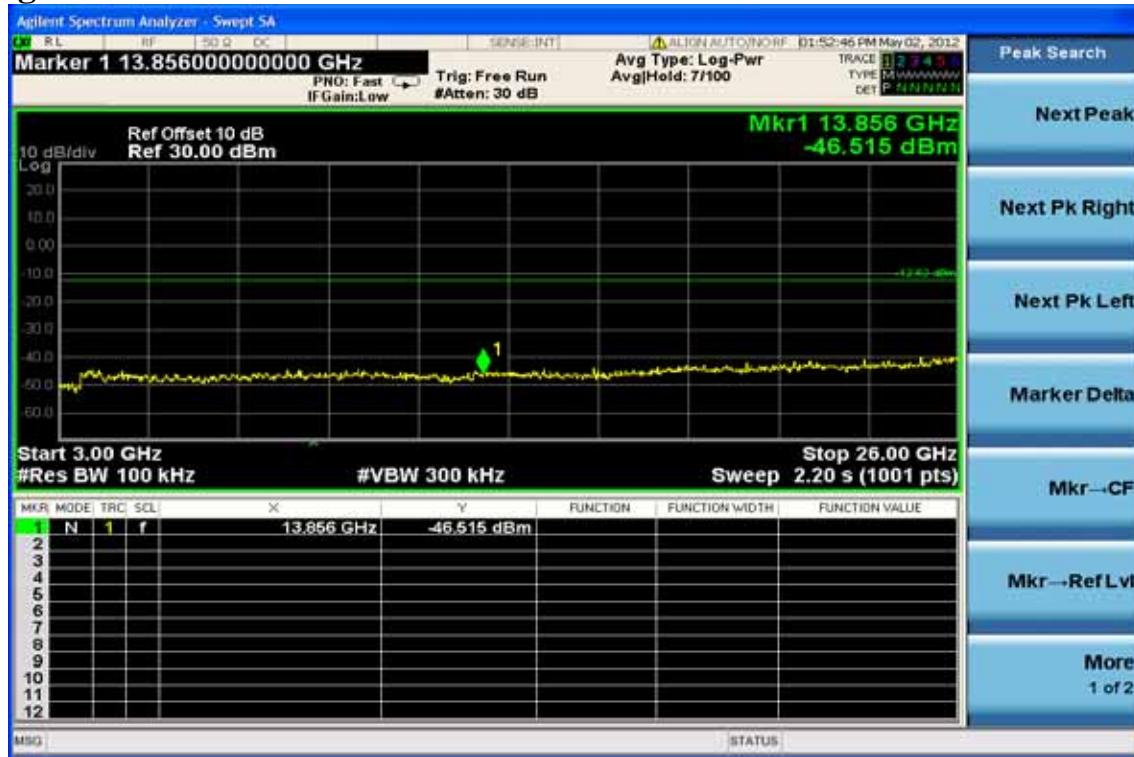
Conducted Spurious Emission Measurement Result (802.11g)
