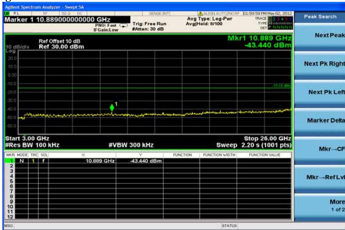
Conducted Spurious Emission Measurement Result (802.11n\_20M)
