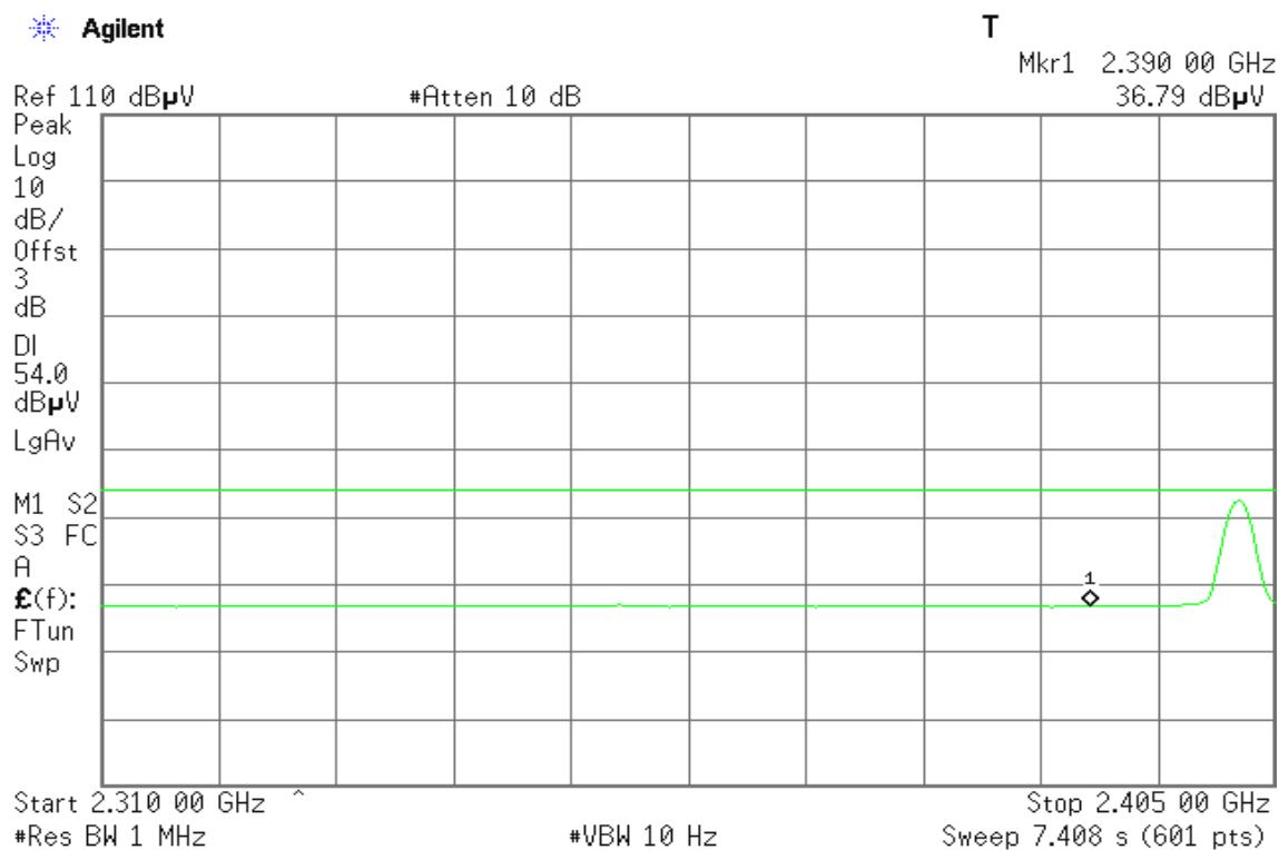
**Band Edges (CH High)****Detector mode: Peak****Polarity: Vertical**
