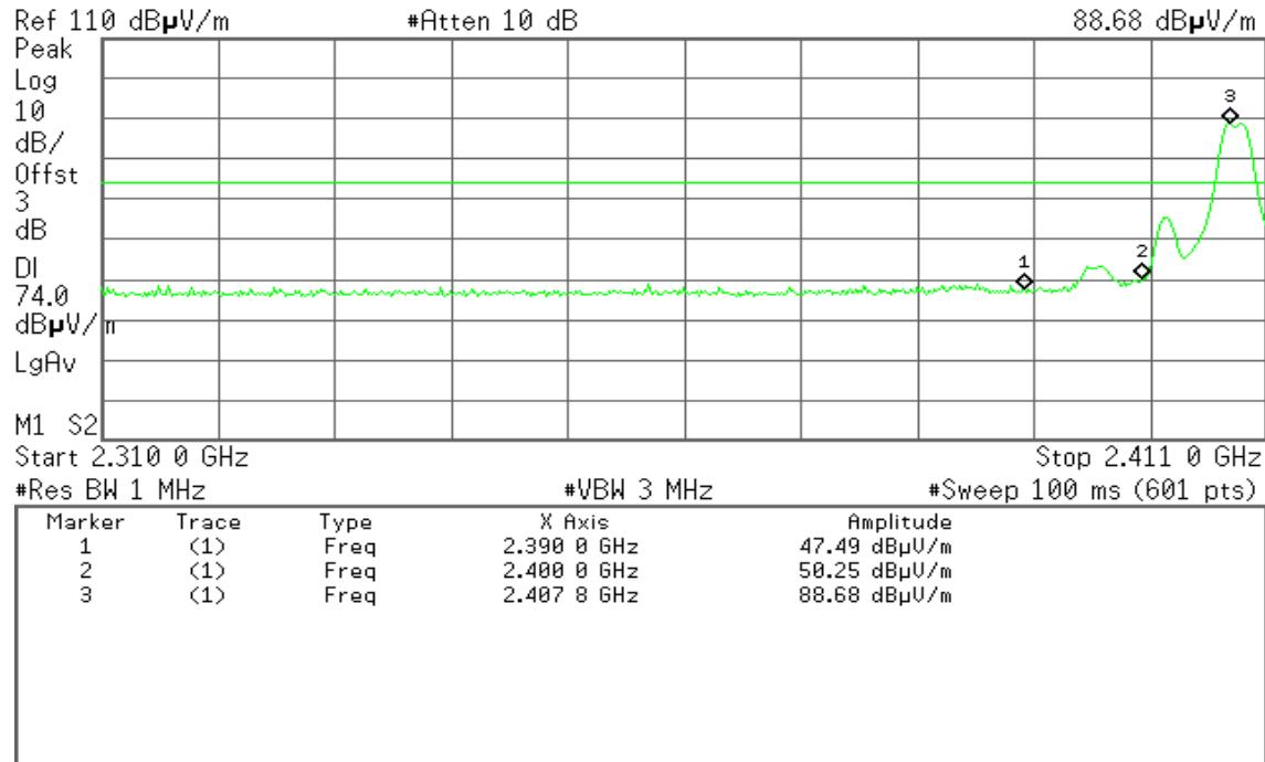
**Detector mode: Average****Polarity: Horizontal****Agilent**
