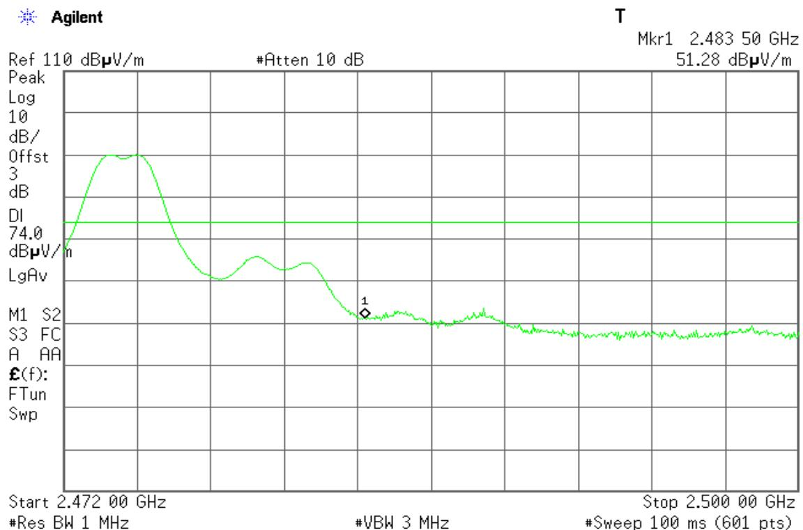
**Detector mode: Average****Polarity: Horizontal**
