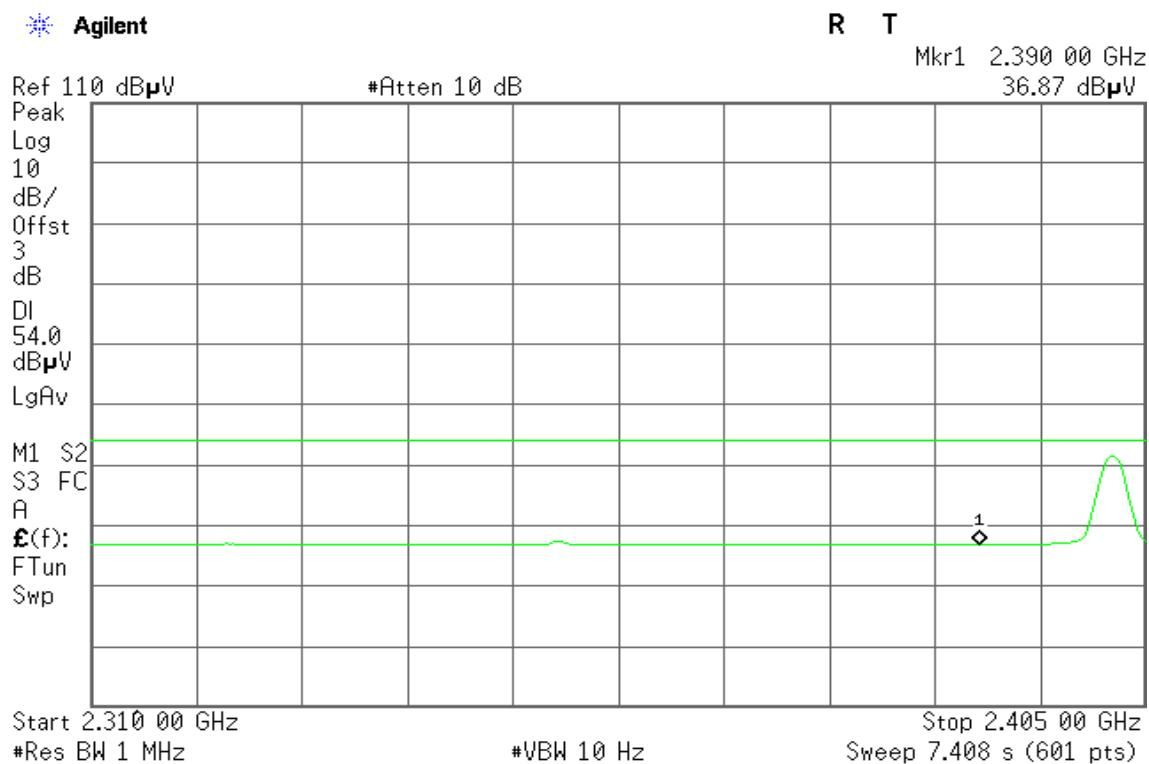
**Band Edges (CH High)****Detector mode: Peak****Polarity: Vertical**
