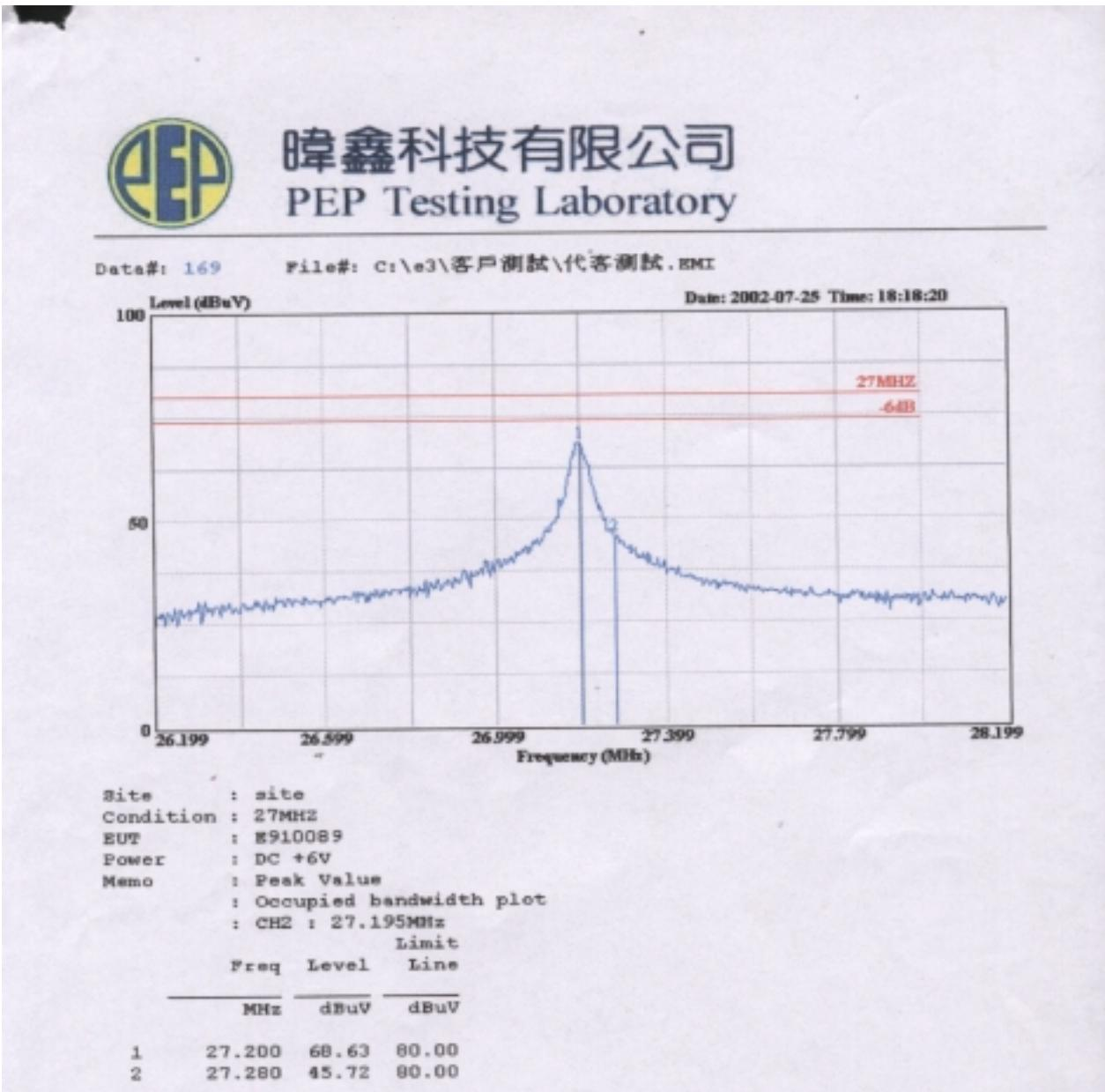
Limit (3m) = 49.54dB $\mu$ V/m∴ 45.72 dB $\mu$ V < Limit
