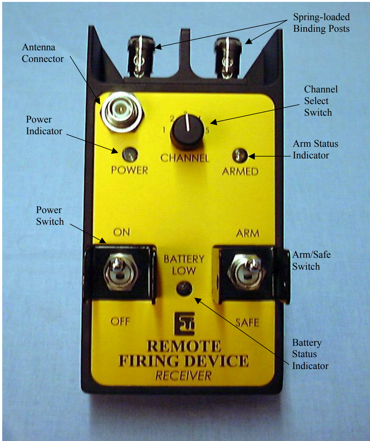
Figure 2. RFD receiver unit controls and indicators.
