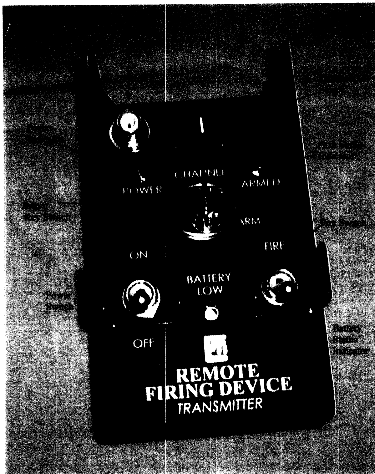
Figure 6. RFD transmitter unit controls and indicators.
