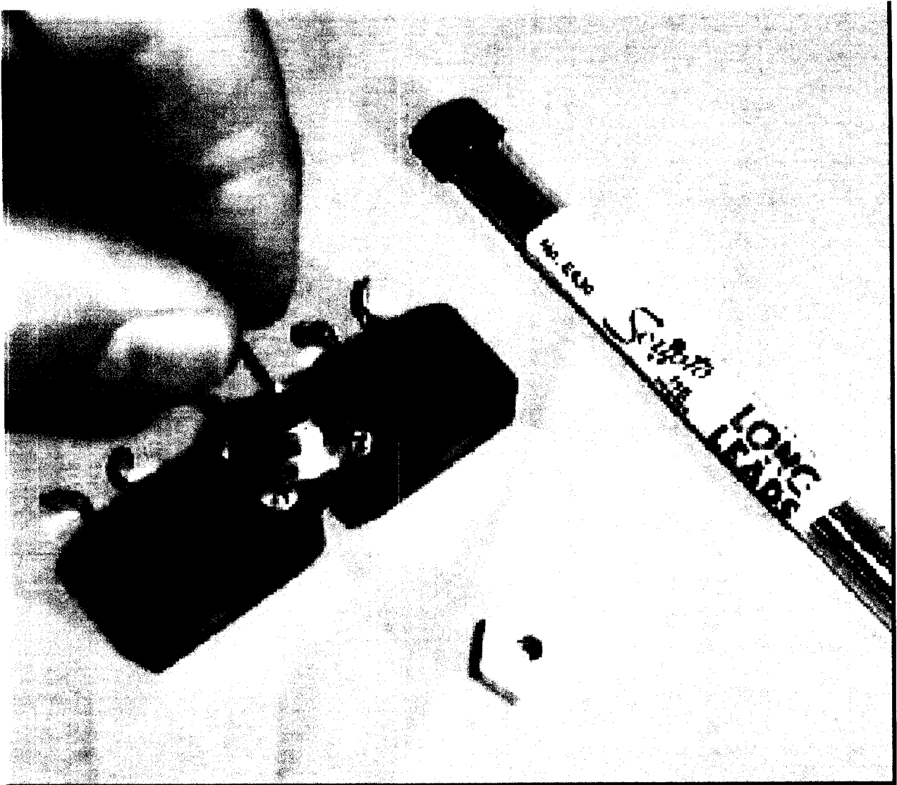
Figure 11. Spark igniter re-carbonizing procedure.
