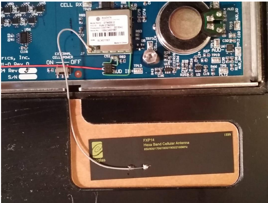
Cellular module and antenna detail, with adhesive removed
