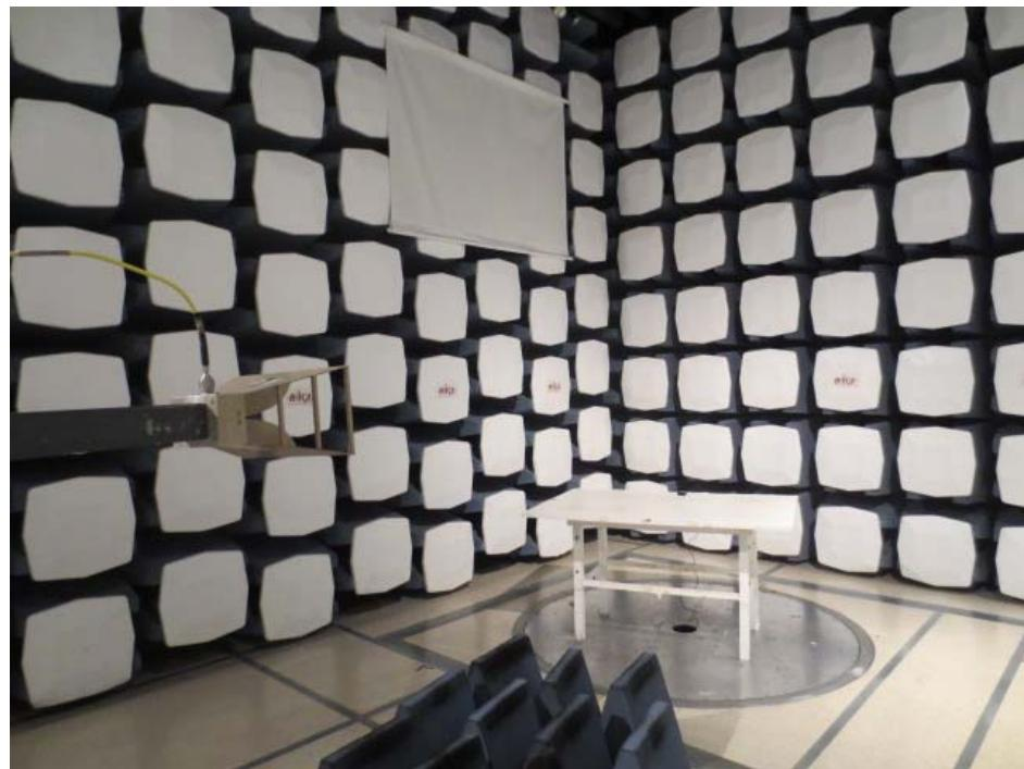
**16.4 Radiated Emission Above 1 GHz Rear View at 3 Meter**
