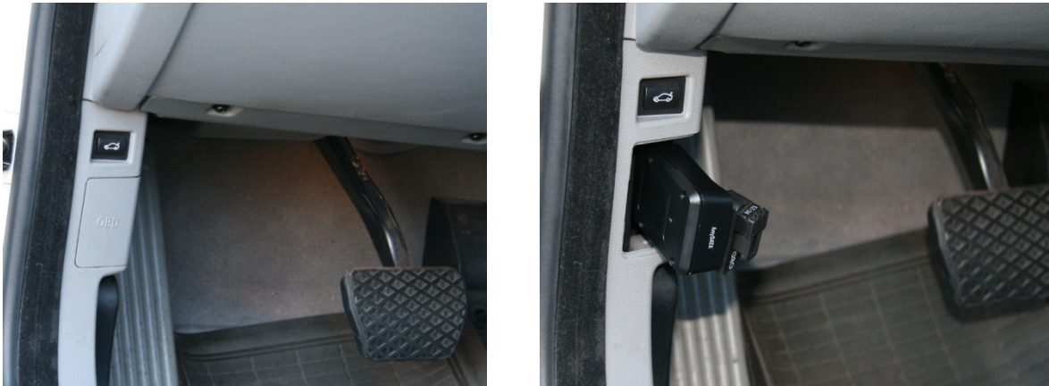
Figure 4.1: Installation of ACT10 in vehicle
