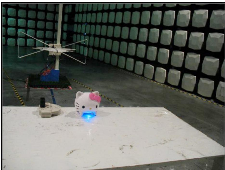
Above 1GHz:(full anechoic chamber)
