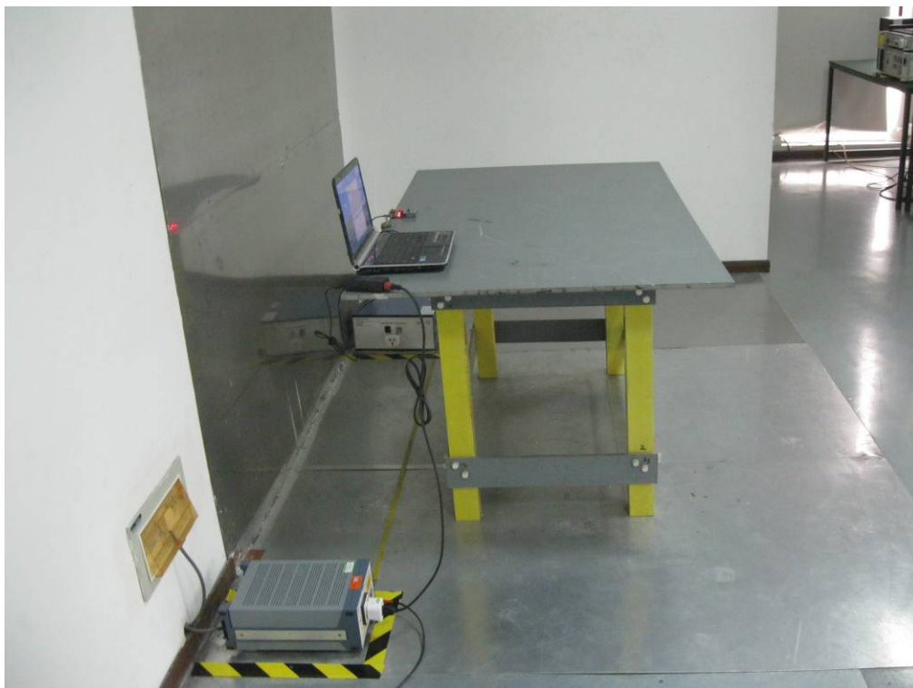
Conducted Emissions Test Setup Side View
