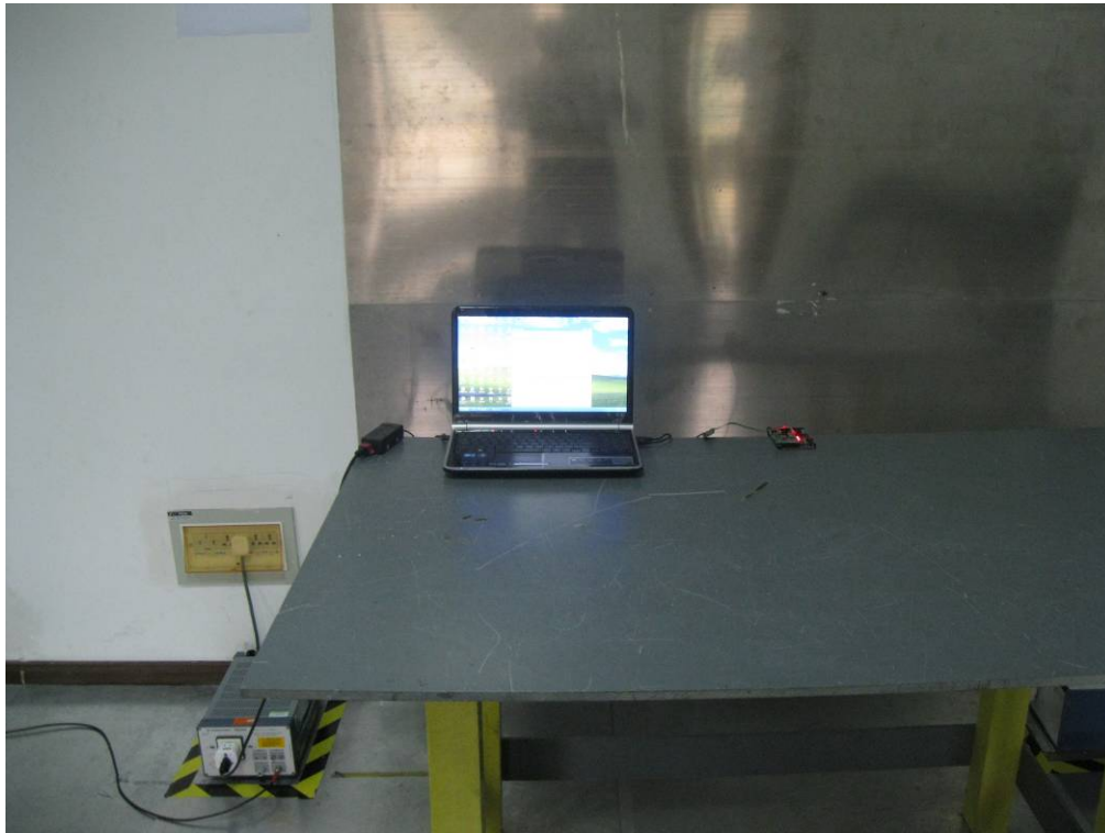
Conducted Emissions Test Setup Front View
