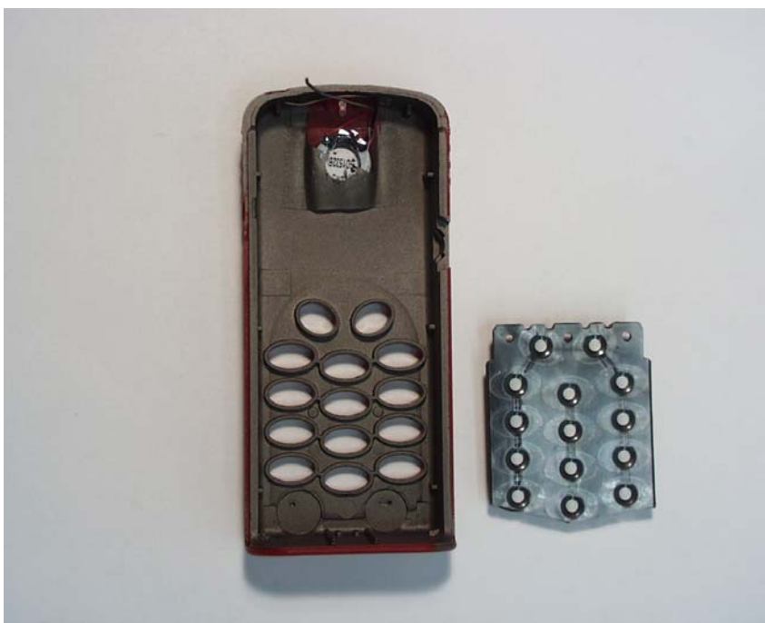
< EMI/RFI shielding spray had been applied to the inner side of the front case >
