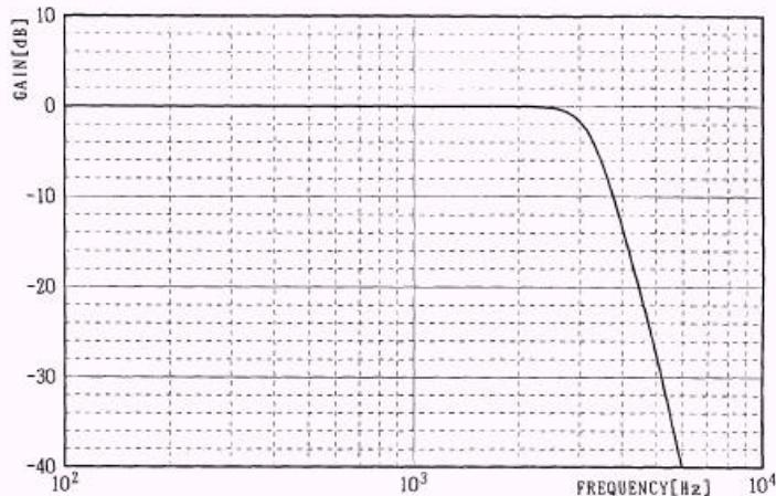
Fig - 3 Frequency Response of Splatter Filter
