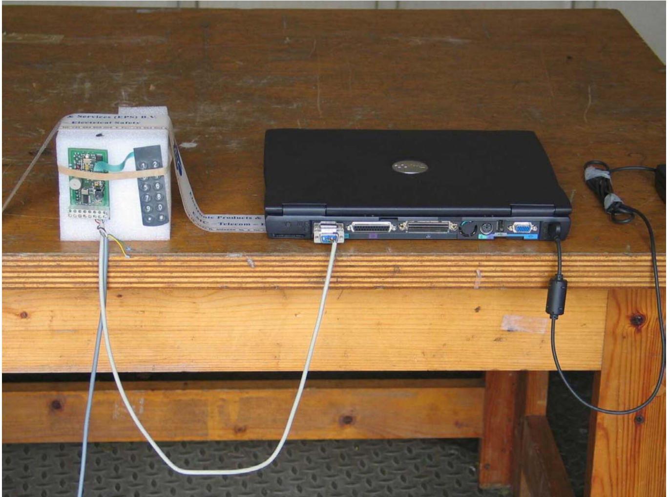
Photo 1: close up radiated emission measurements.
