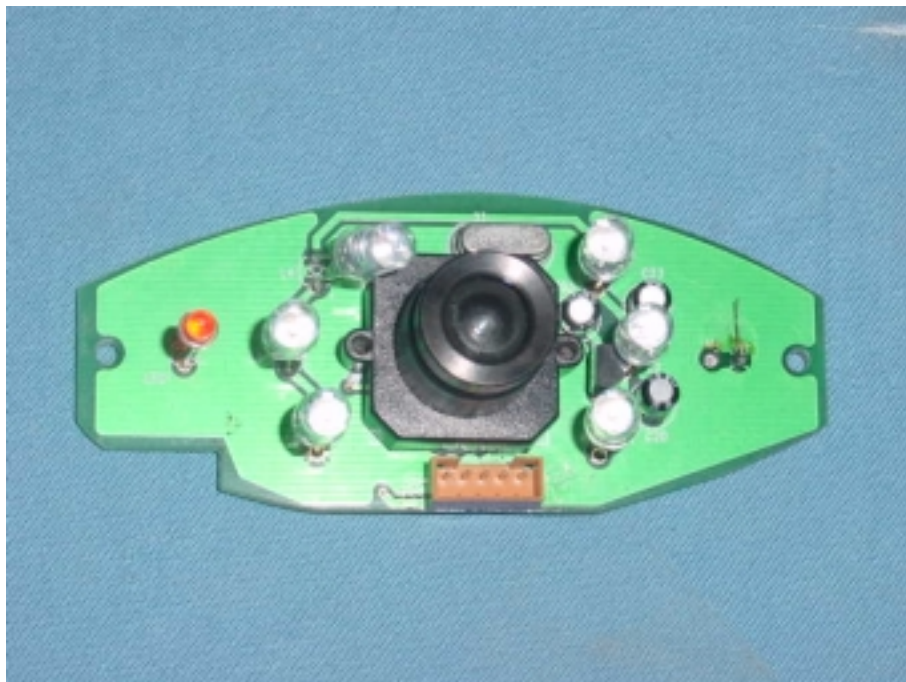
Figure 6 Main Board, Component Side
