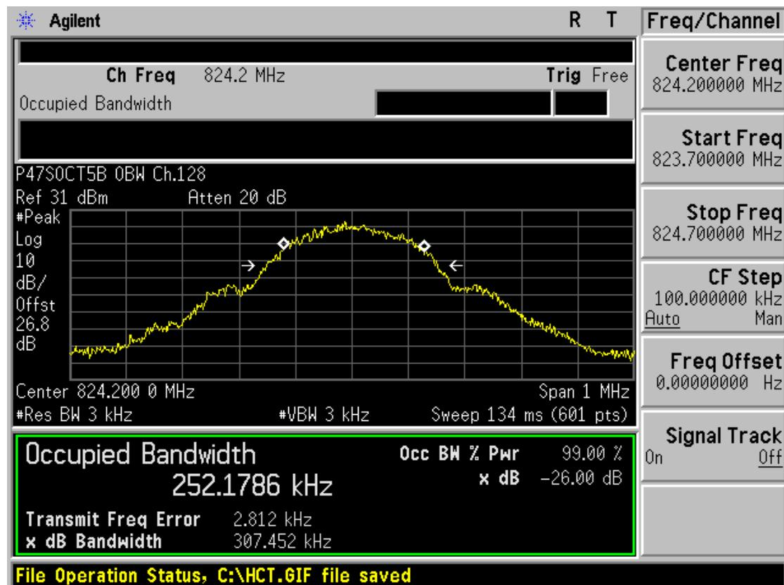
■ GSM850 MODE (190 CH.) Occupied Bandwidth
