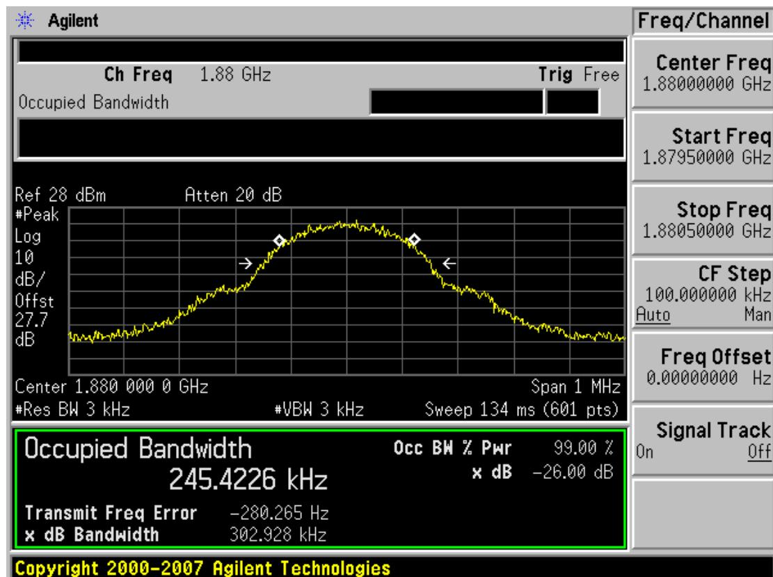
■ GSM1900 MODE (810 CH.) Occupied Bandwidth
