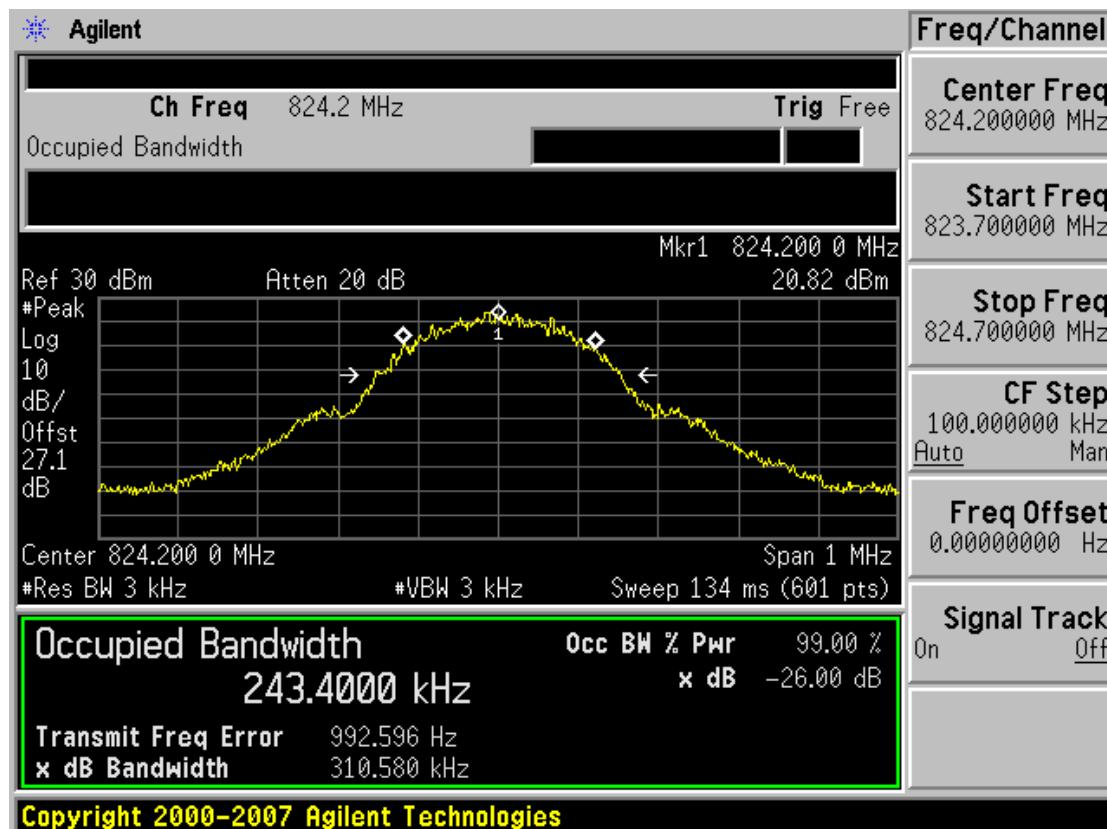
■ GSM850 MODE (190 CH.) Occupied Bandwidth
