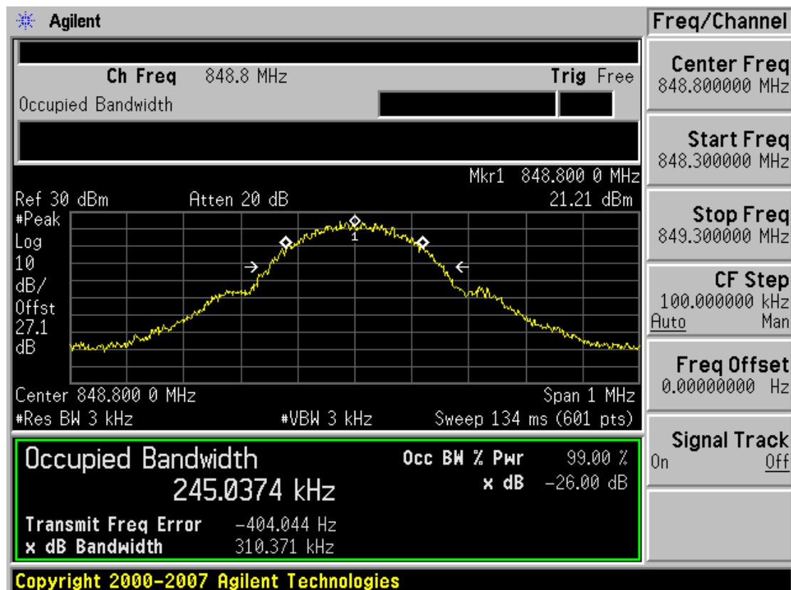
■ GSM1900 MODE (512 CH.) Occupied Bandwidth
