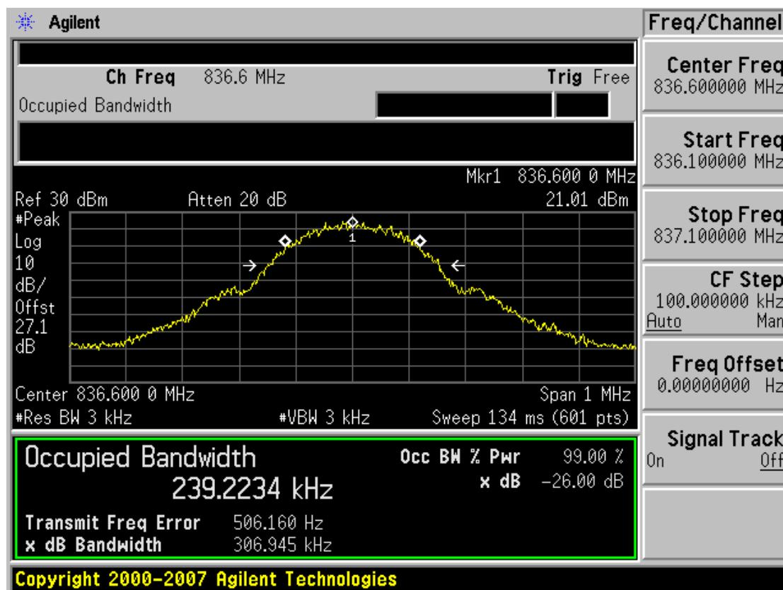
■ GSM850 MODE (251 CH.) Occupied Bandwidth
