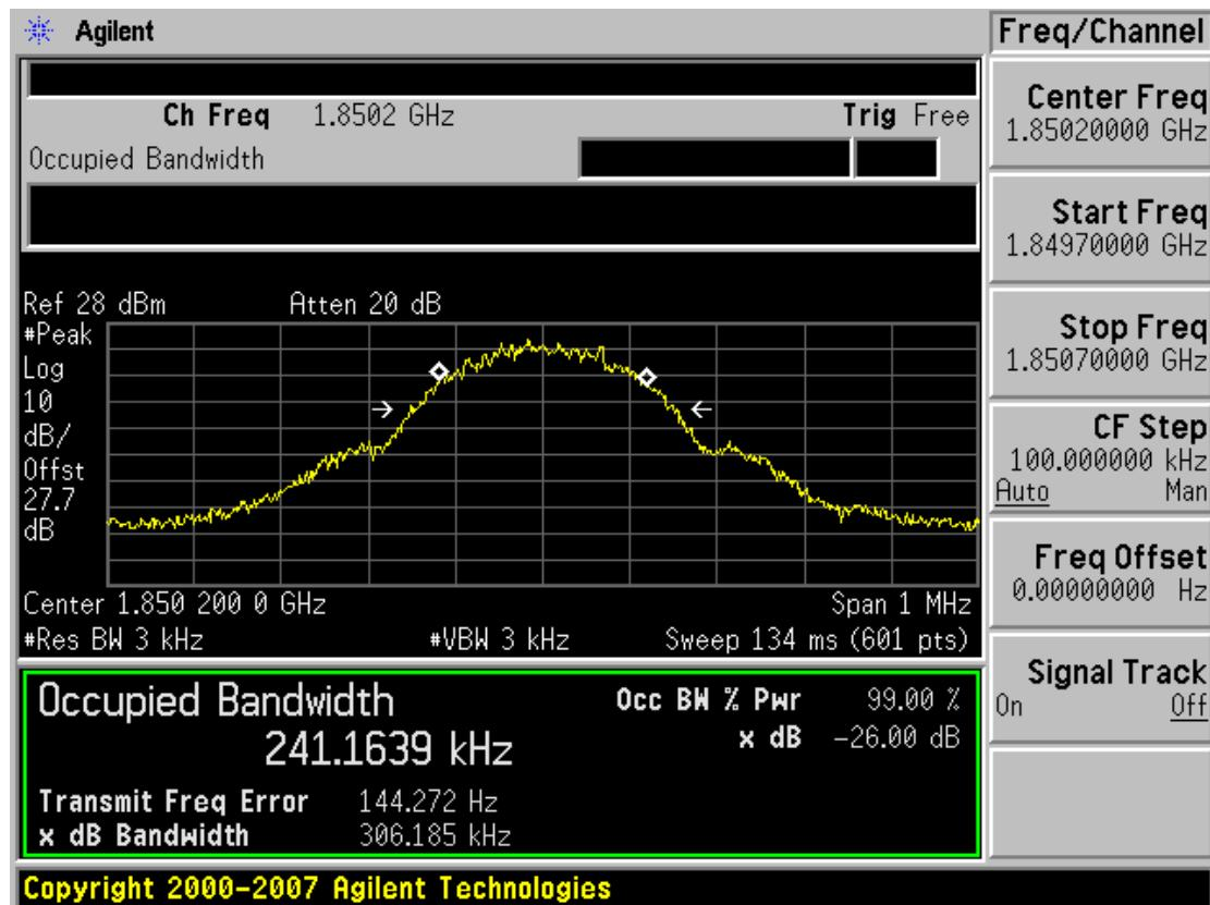
■ GSM1900 MODE (661 CH.) Occupied Bandwidth
