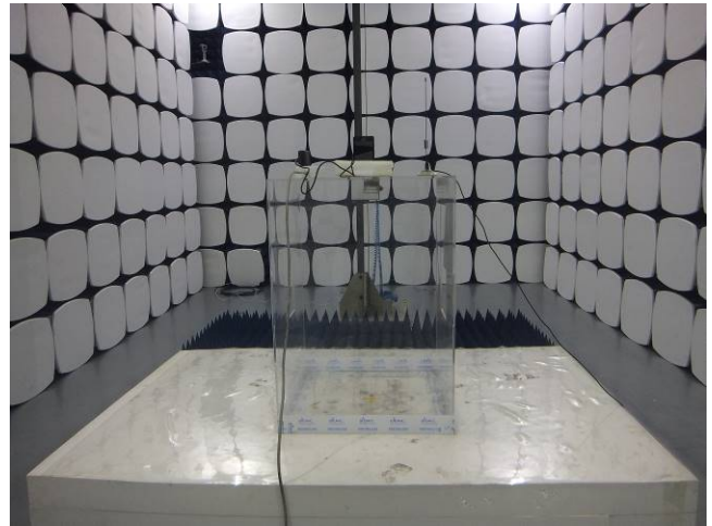
Radiated Spurious Emissions Test Setup Above 1GHz
