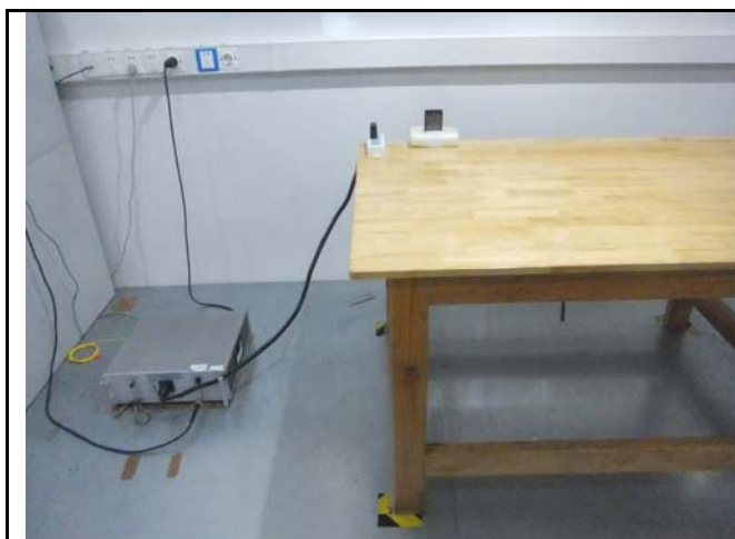
Conducted Emissions Test Setup Front View
