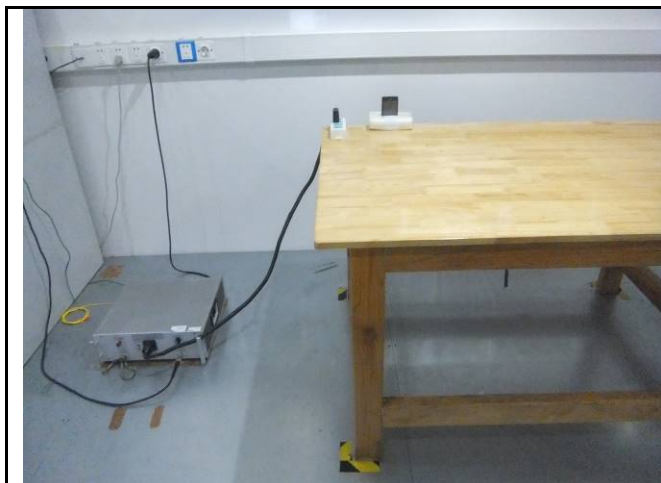
Conducted Emissions Test Setup Front View
