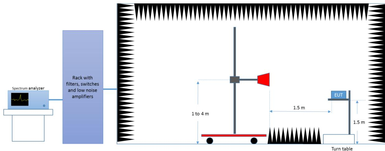
Test Results – GSM850**GSM850 GPRS/GMSK - Low Channel CH128****Radiated Spurious – 30MHz to 40GHz**
