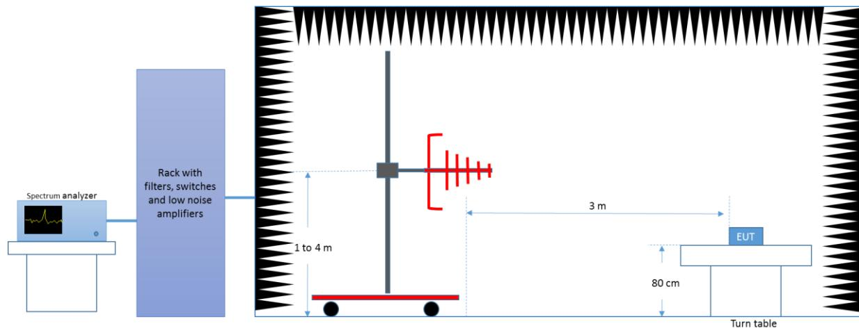
*Radiated Setup Frequency range 1GHz - 18GHz*
