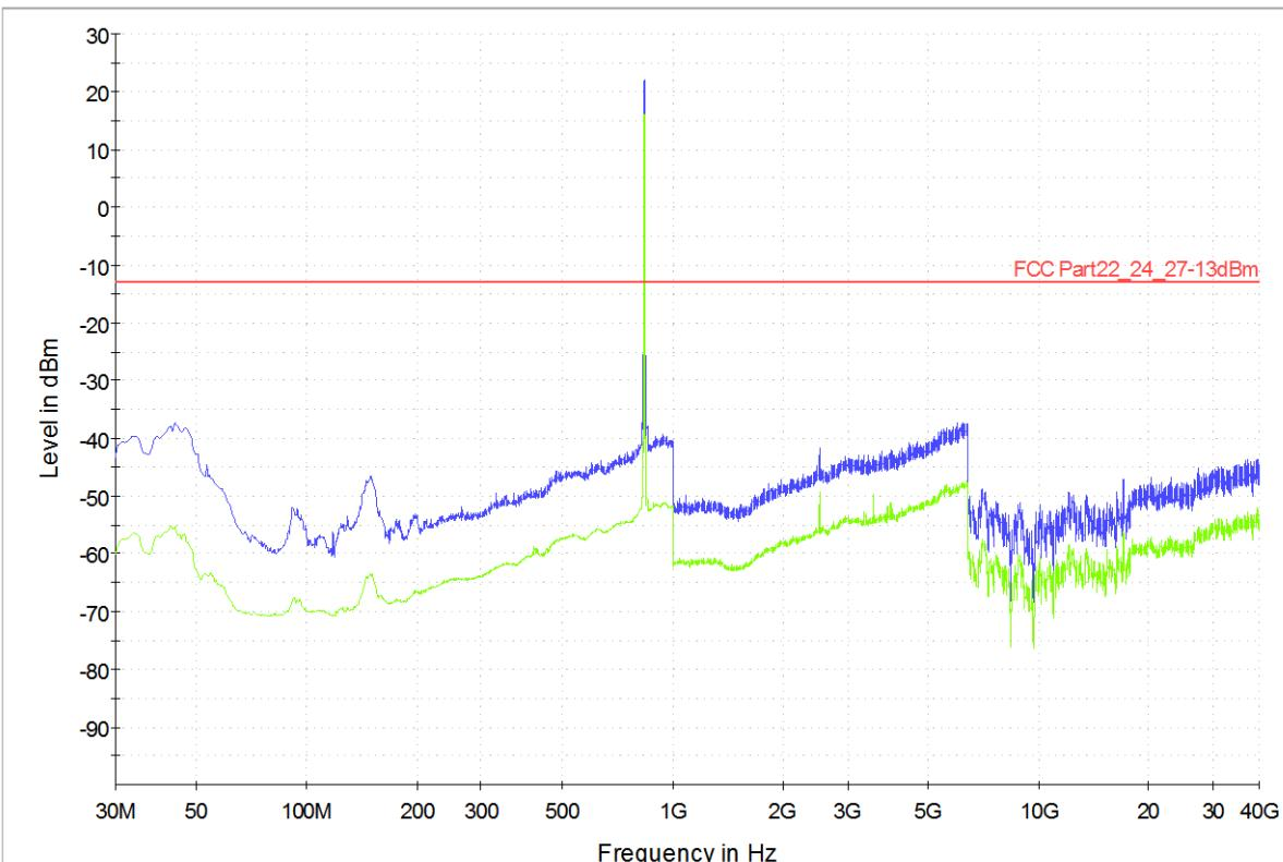
— Peak measurements      — RMS measurements      — Limit FCC
