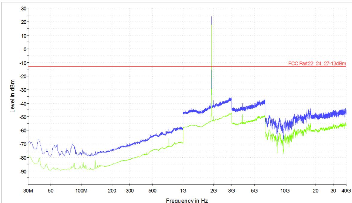
— Peak measurements      — RMS measurements      — Limit FCC
