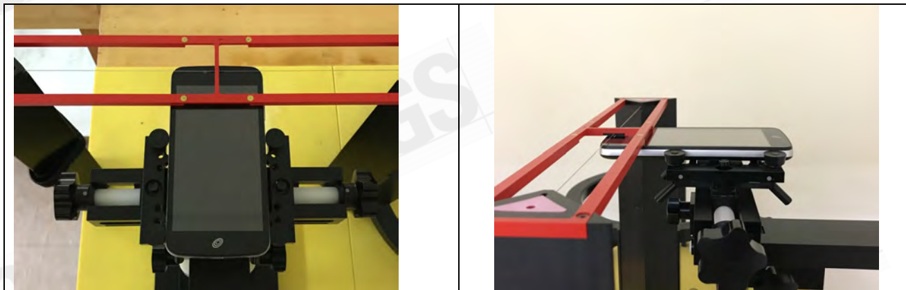
Fig. 1 Photograph of the DASY 5 measurement system
