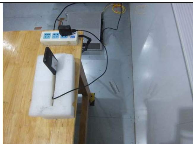
Conducted Emissions Test Setup Side View
