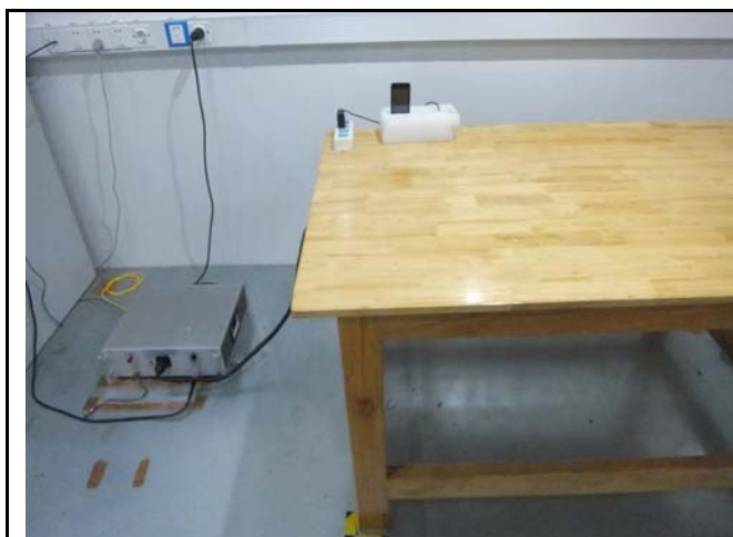
Conducted Emissions Test Setup Front View
