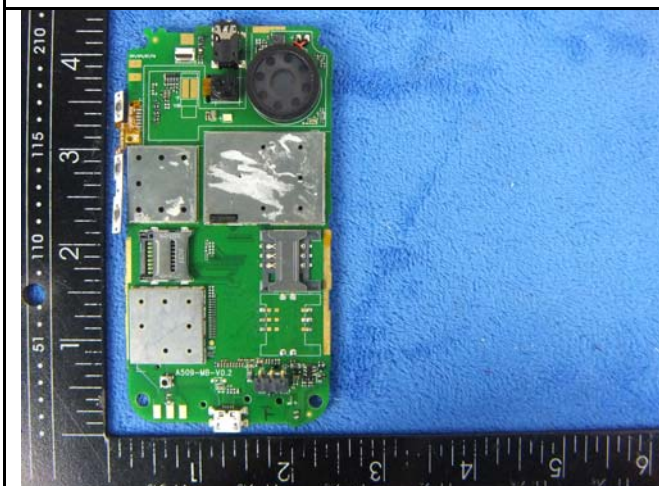
Mainboard with Shielding - Front View
