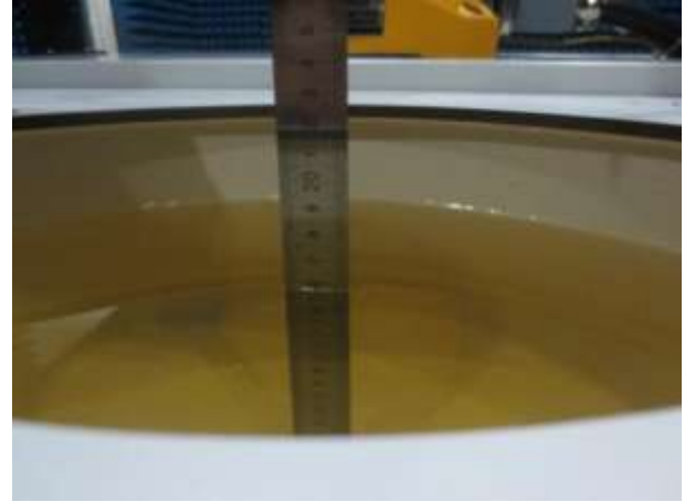
Fig. 9.2 Photo of Liquid Height for Body SAR
