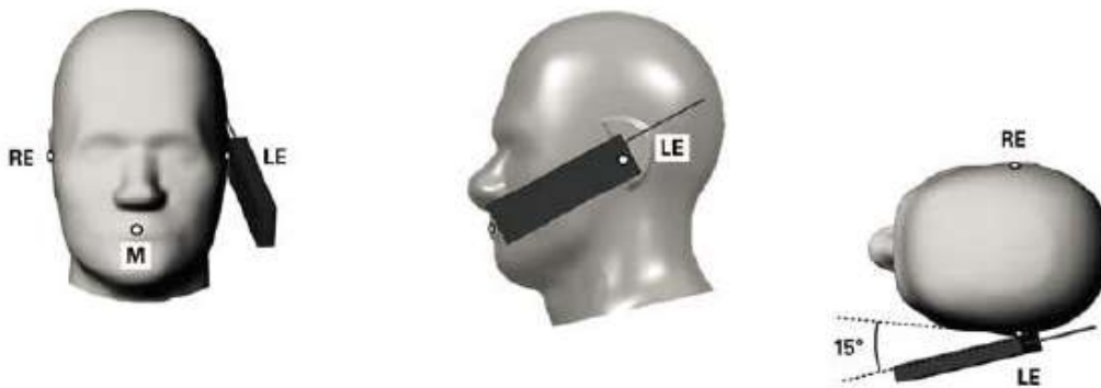
Fig.11.4 Illustration for Tilted Position
