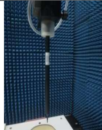
Fig. 8.2 Photo of E-Field Probe
