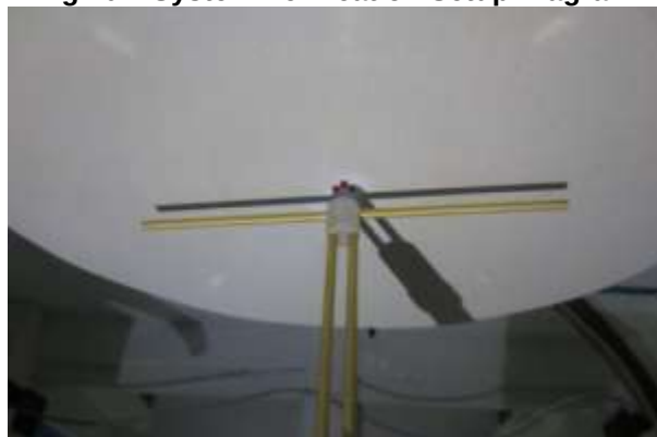
Fig.10.2 Photo of Dipole setup
