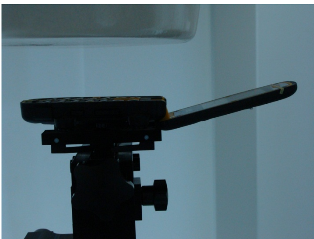
Right Cheek position - Separation distance 4.2cm between mouth and antenna
