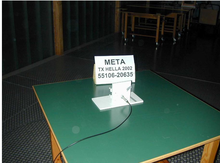
Test setup for radiated emission final test 30 MHz - 1 GHz
