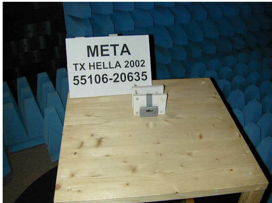
Test setup for radiated emission pre-test 30 MHz - 1 GHz and final test 1 GHz to 5 GHz
