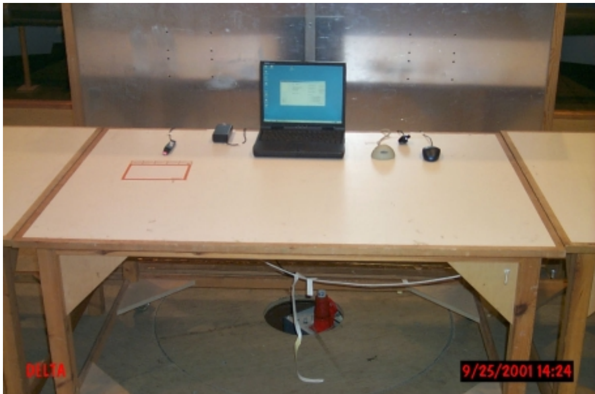
PHOTO A2.1 AC mains conducted emission measuring
