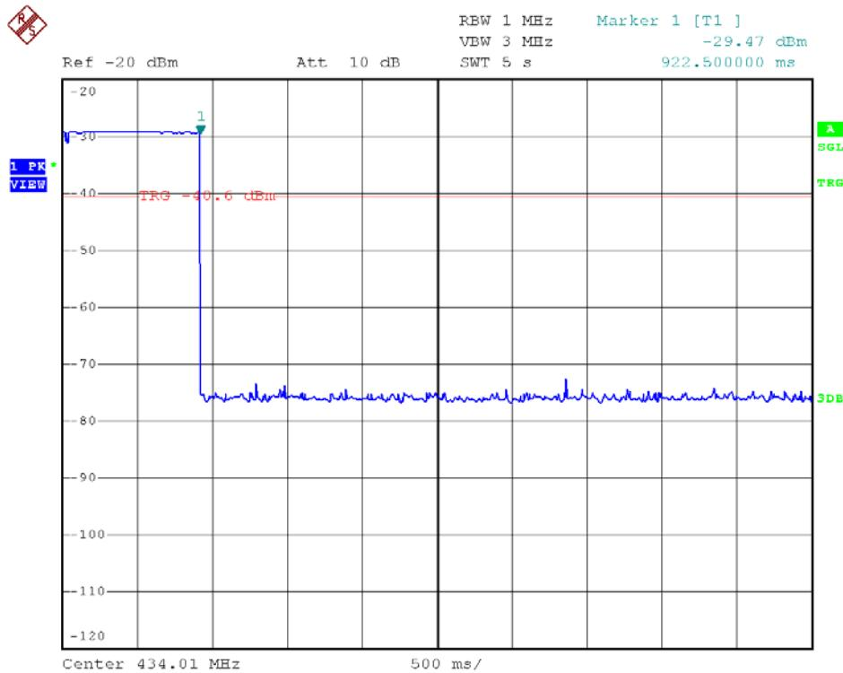
Timing Plot – Pursuant to FCC Part 15 Section 15.231 (a) Requirement
