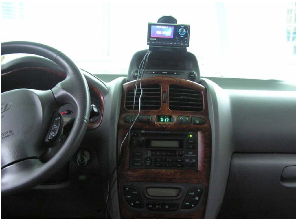
Radiated Emissions(88.10 MHz- 107.90 MHz)- Install
