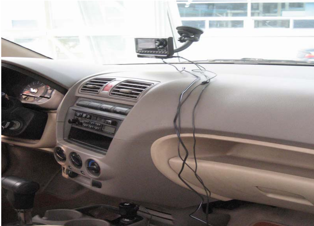
Radiated Emissions(88.10 MHz- 107.90 MHz)- Install
