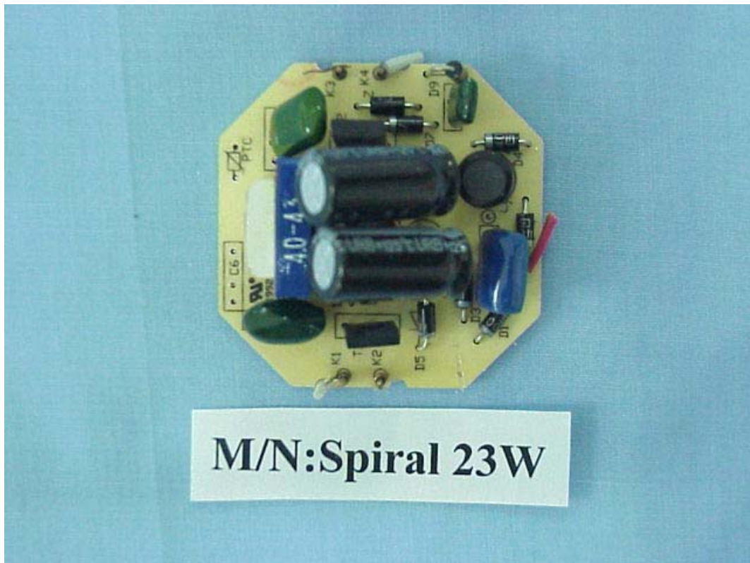
FIGURE 5 LIGHT(M/N: SPIRAL-23W) MAIN BOARD (COMPONENT SIDE)
