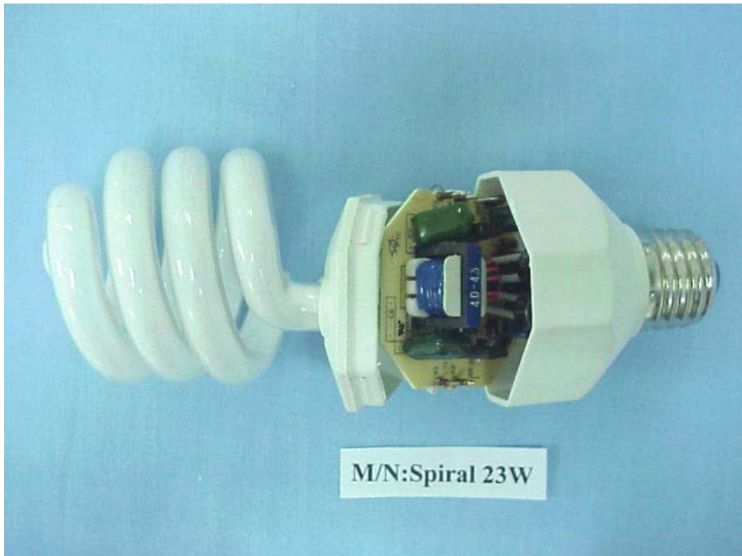
FIGURE 4 LIGHT(M/N: SPIRAL-23W) COVER REMOVED
