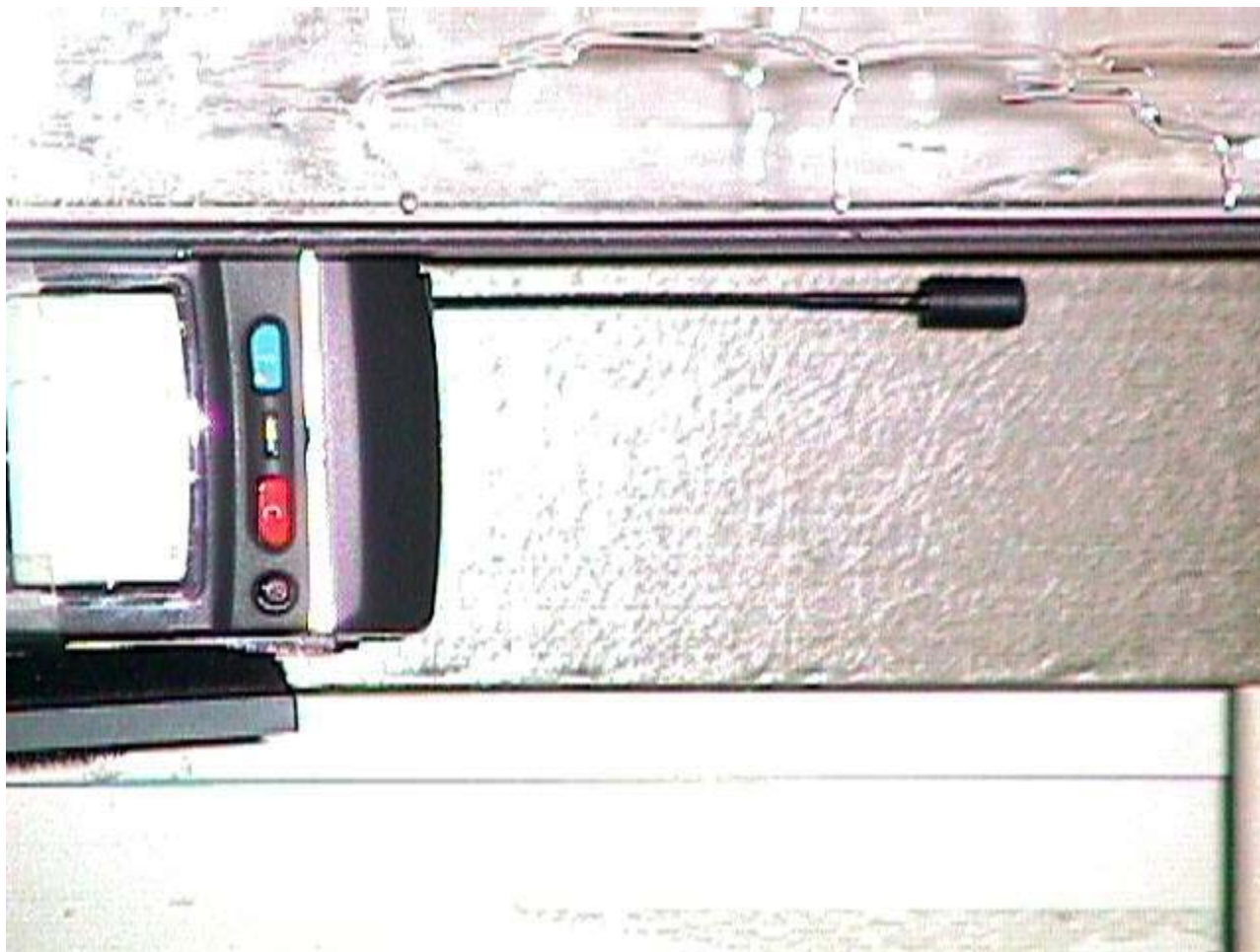
< Right side of EUT faced to the phantom and the antenna fully extended - Close-up view >
