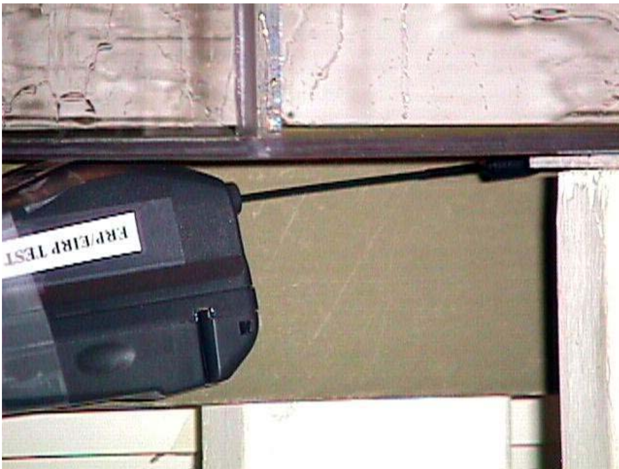
< Back side of EUT faced to the phantom and the antenna fully extended – Close-up Overview >
