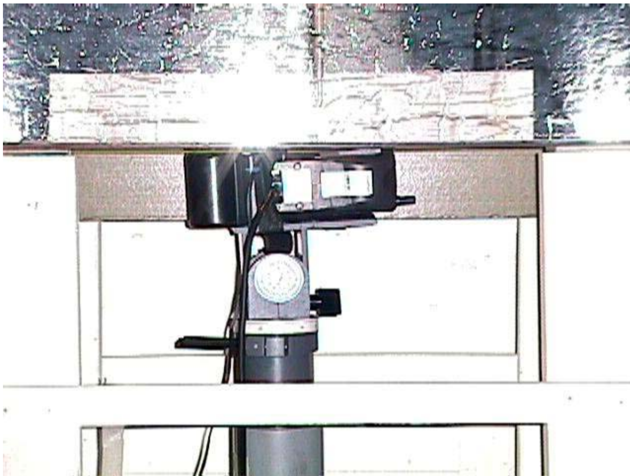
< Left side of EUT faced to the phantom and the antenna fully retracted - Close-up view >
