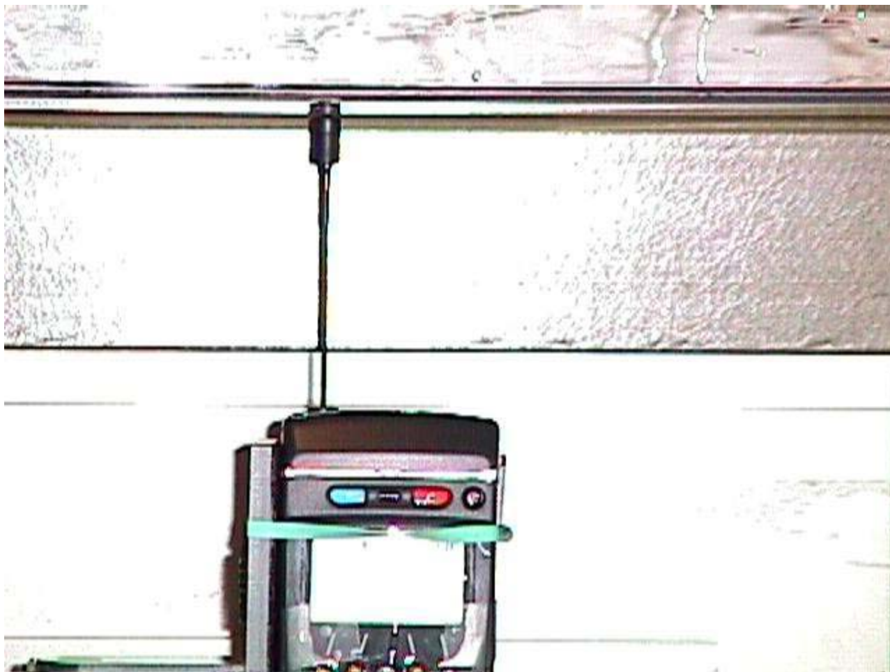
< Top of EUT faced to the phantom and the antenna fully extended – Close-up view >
