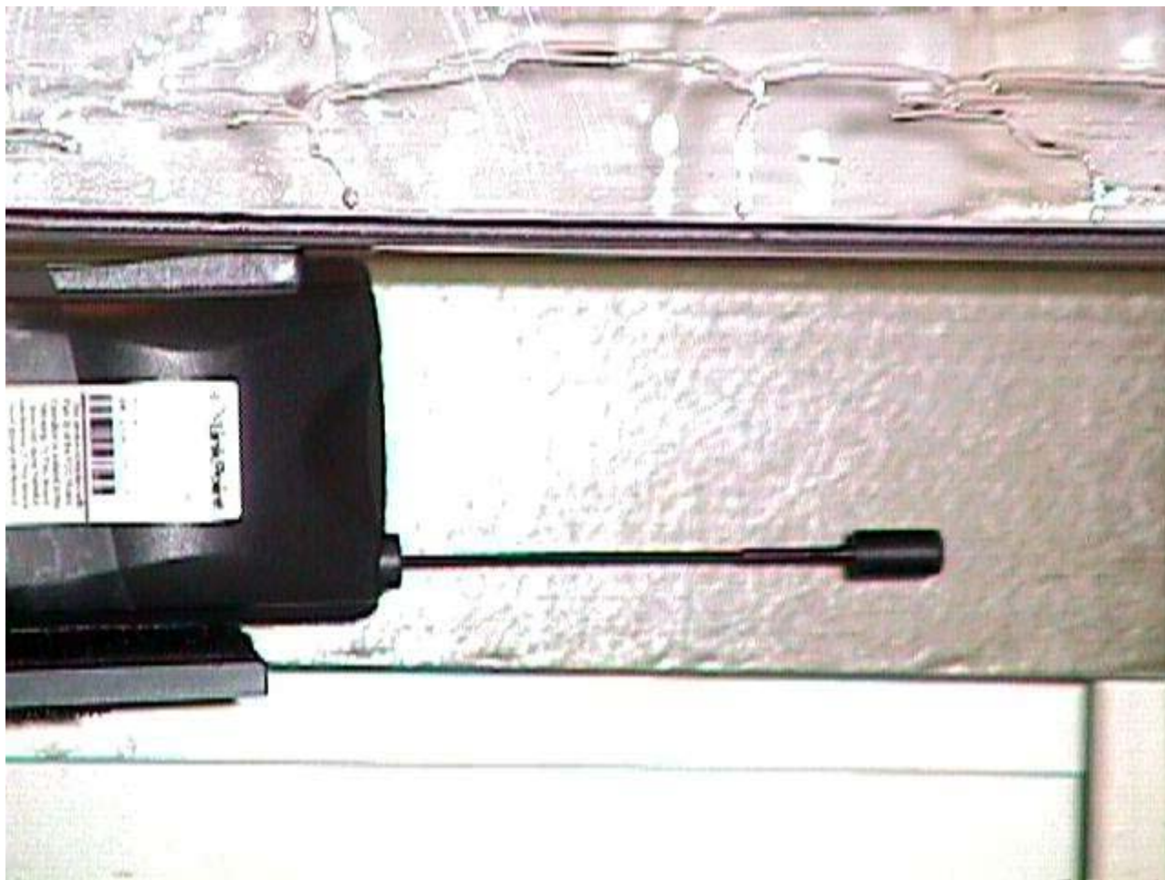
< Left side of EUT faced to the phantom and the antenna fully extended - Close-up view >
