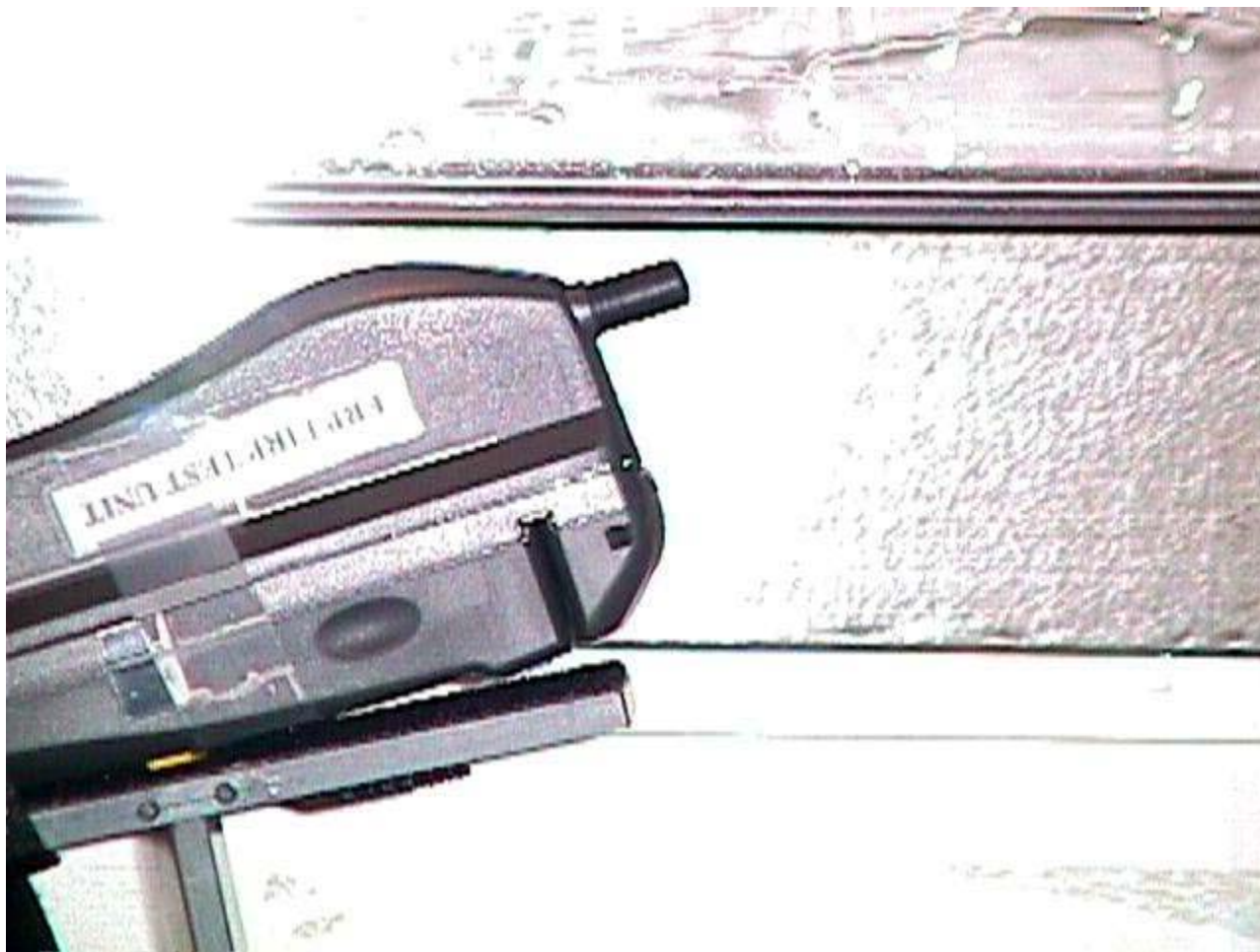
< Back of EUT faced to the phantom at 4 mm separation and the antenna fully retracted – Close-up view >
