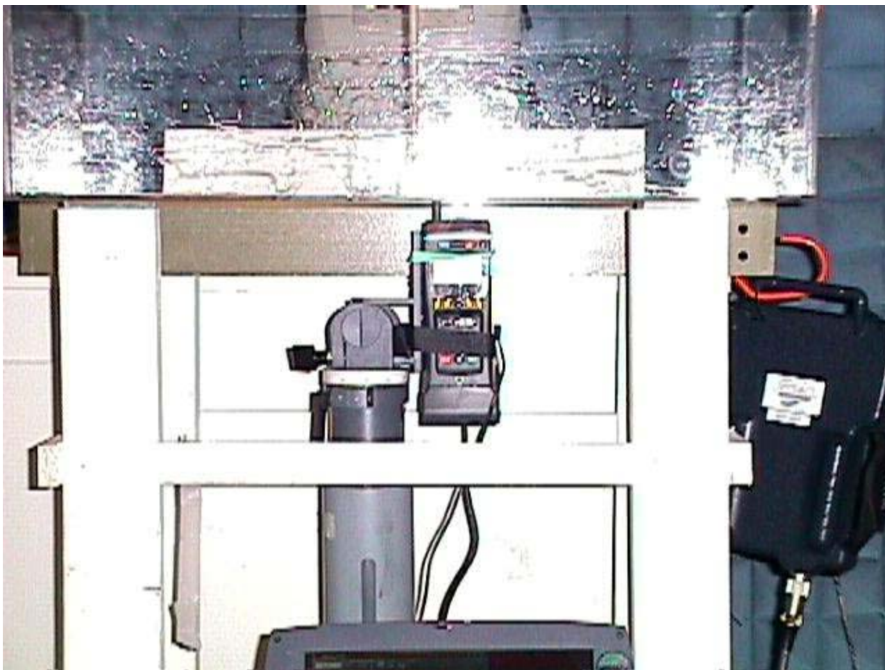
< Top of EUT faced to the phantom and antenna fully retracted – Overview >
