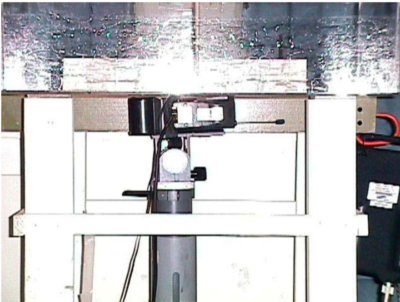
< Left side of EUT faced to the phantom and the antenna fully extended - Overview >
