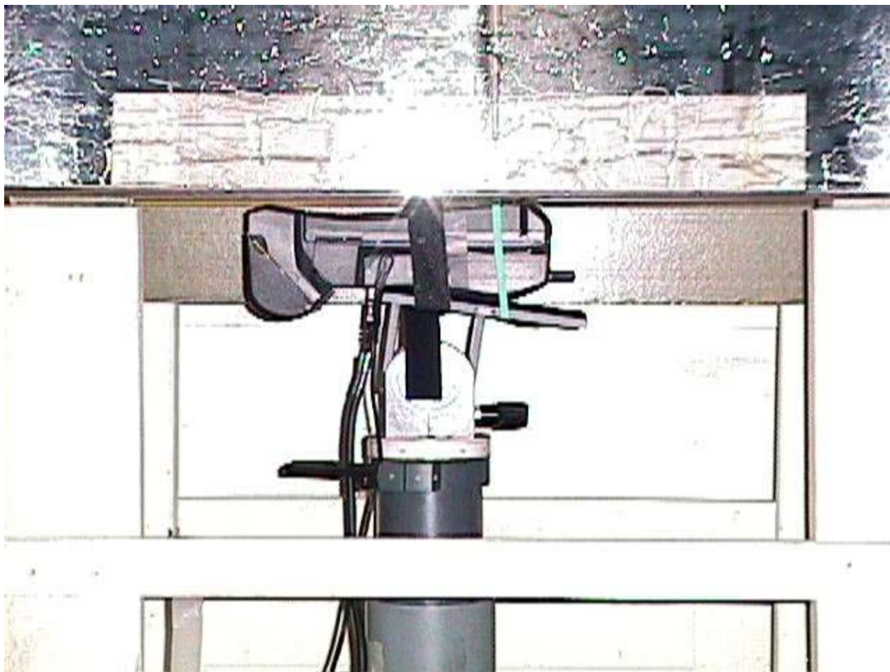
< Front side of EUT faced to the phantom and the antenna fully retracted – Overview >
