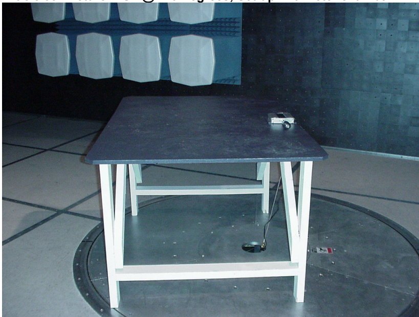
Article 35- Picture: EUT @ 270 Degrees; Set-up in 3-meter chamber
