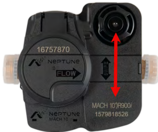
Figure 22 – MACH 10® R900™ with Arrow Showing Direction of Magnet Swipe
