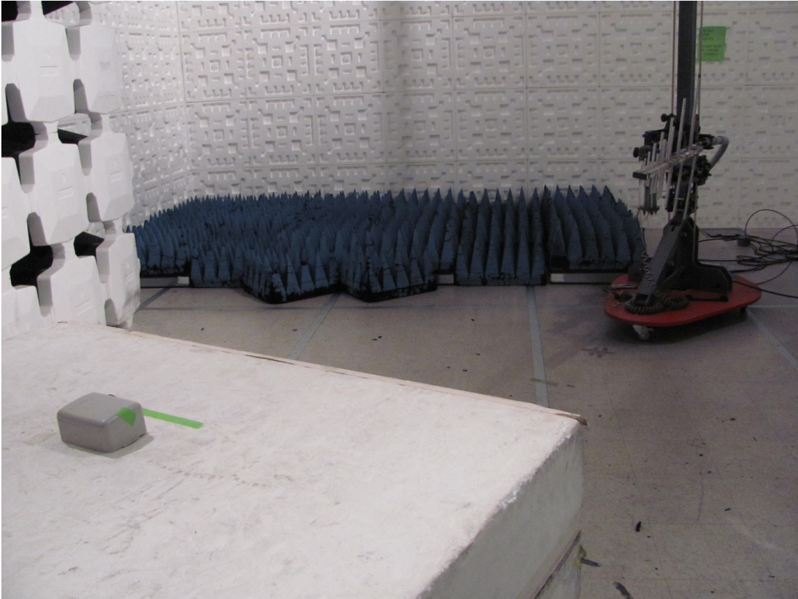
Figure 4. Radiated Emissions, 200-1000 MHz
