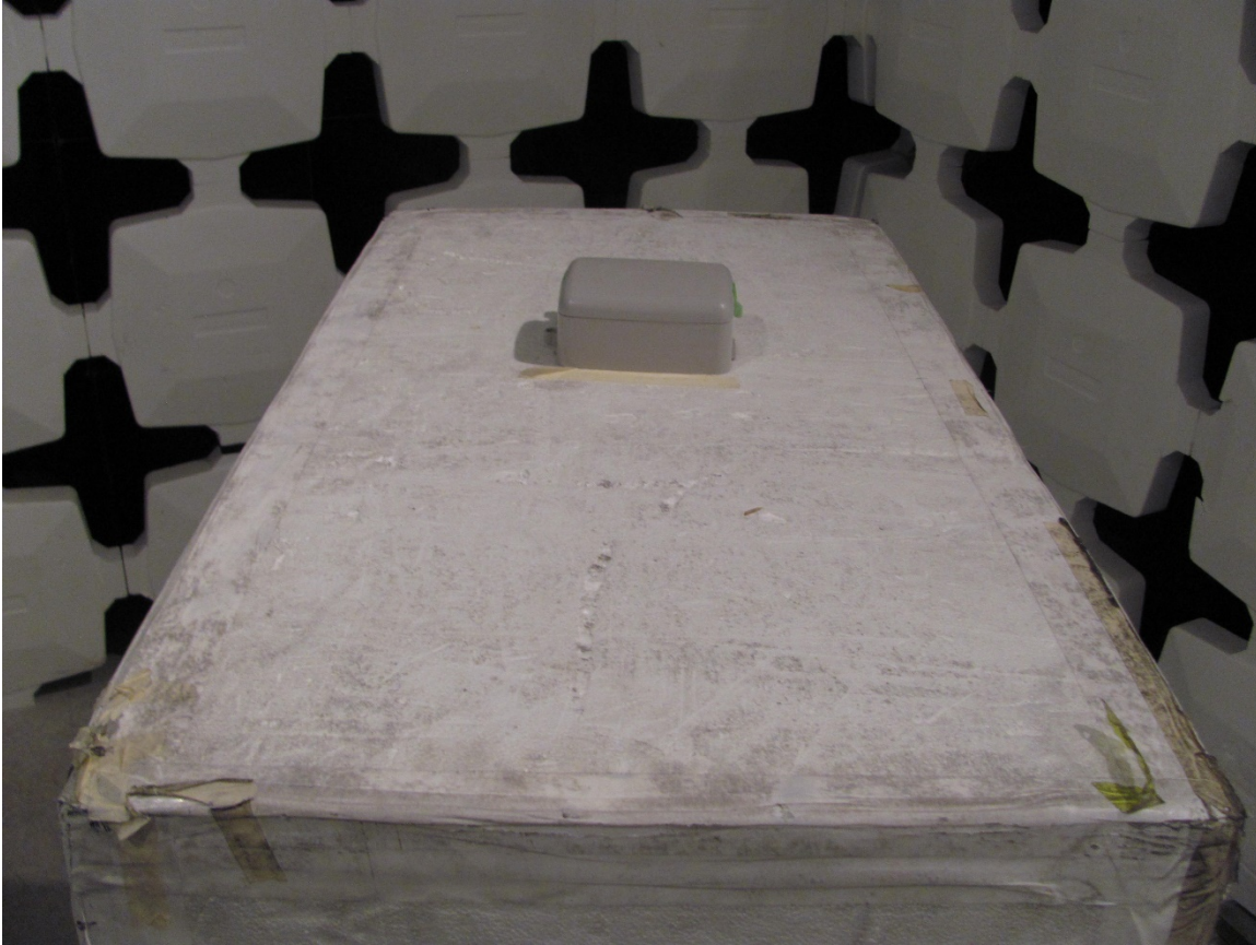
Figure 2. Internal Antenna EUT Setup
