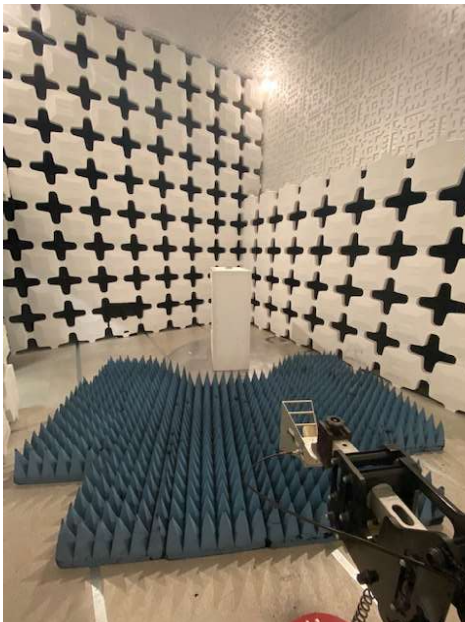
Figure 9. Intentional Radiated Emissions Test Configuration (Above 1 GHz), Internal Antenna
