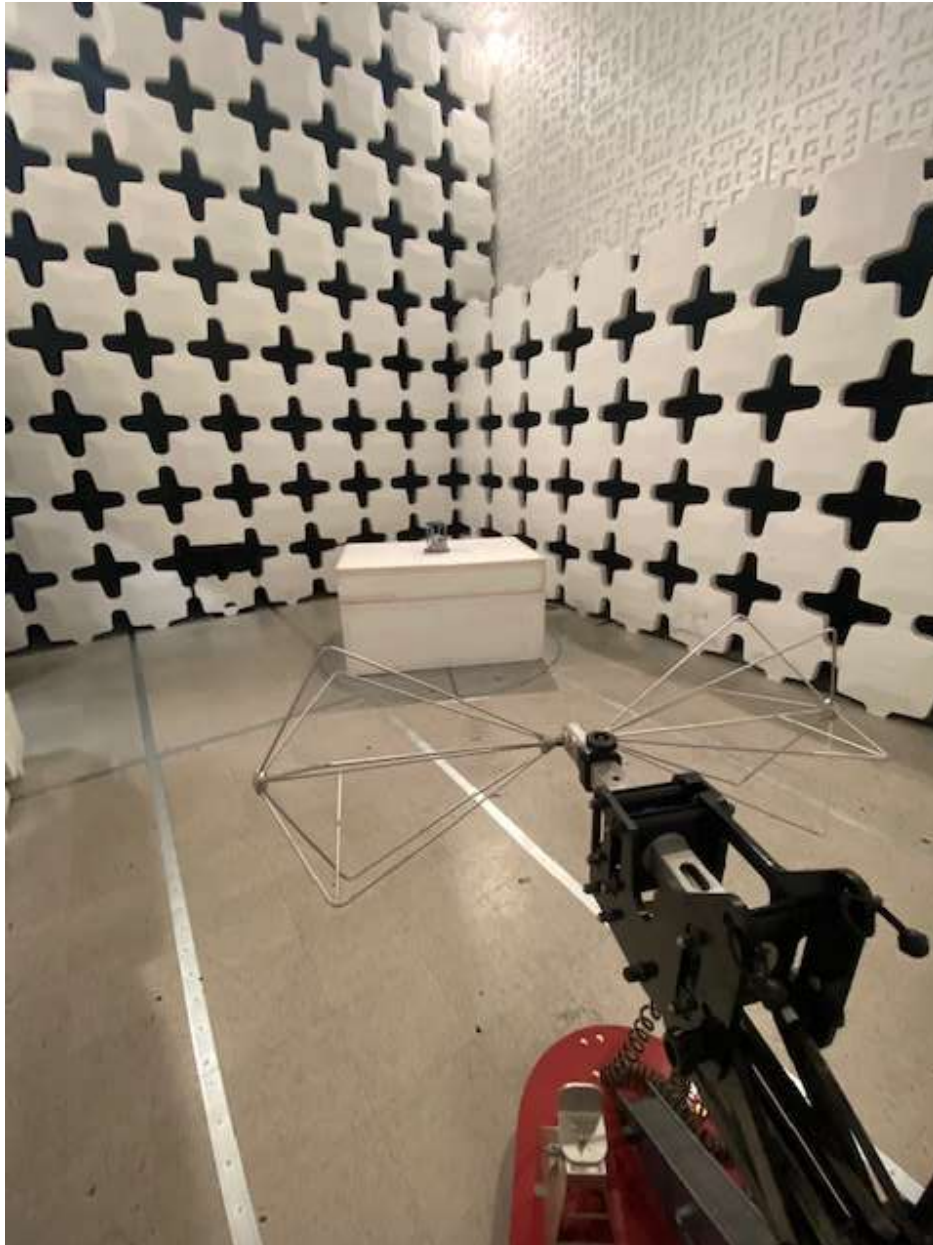
Figure 6. Radiated Emissions Test Configuration (30-200 MHz), External Antenna
