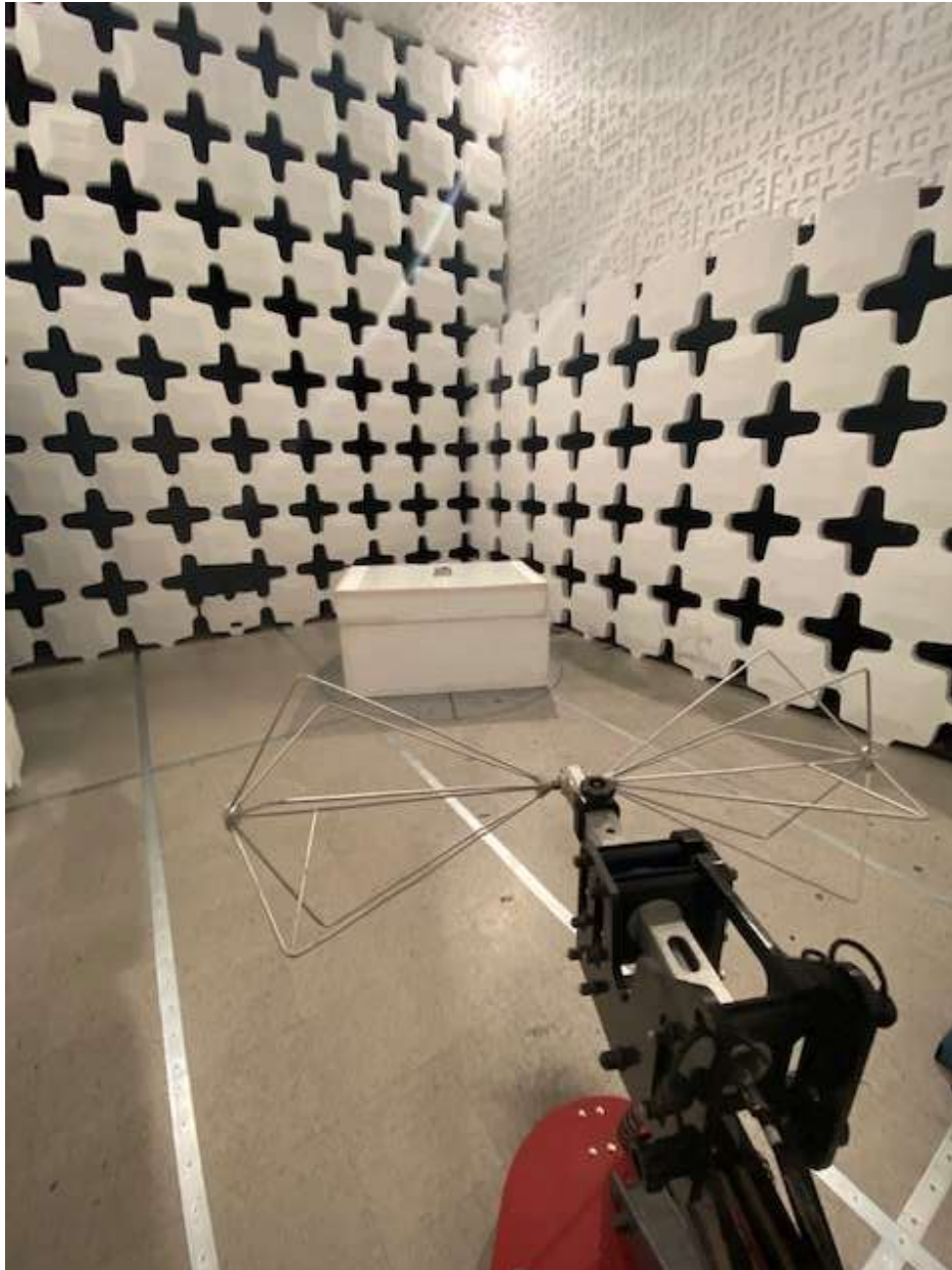
Figure 5. Radiated Emissions Test Configuration (30-200 MHz), Internal Antenna
