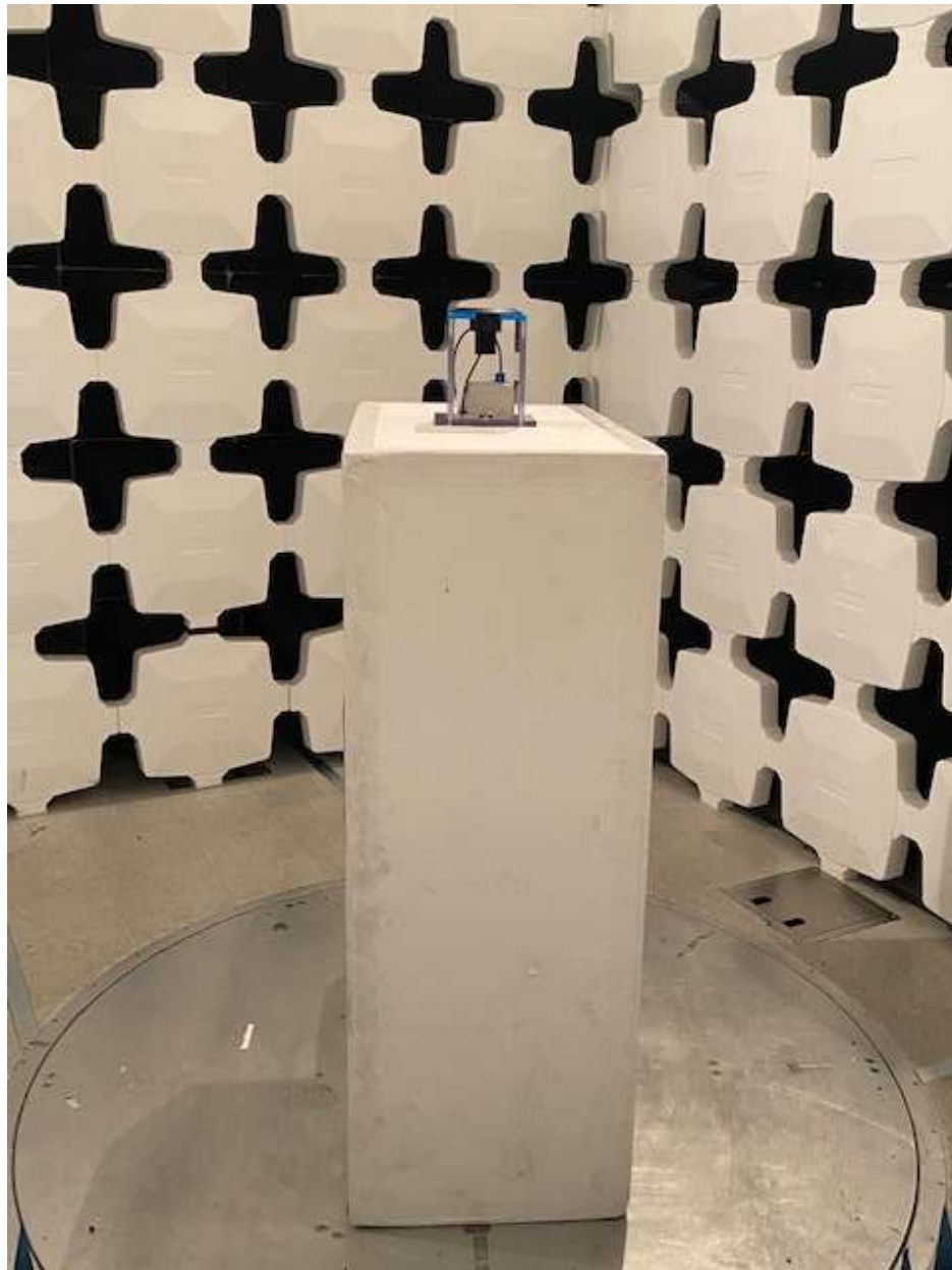
Figure 2. Radiated Emissions Test Setup External Antenna
