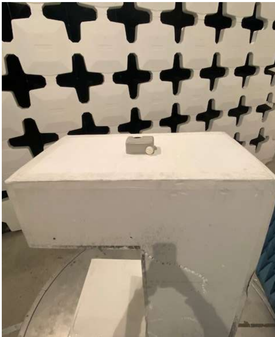
Figure 1. Radiated Emissions Test Setup Internal Antenna
