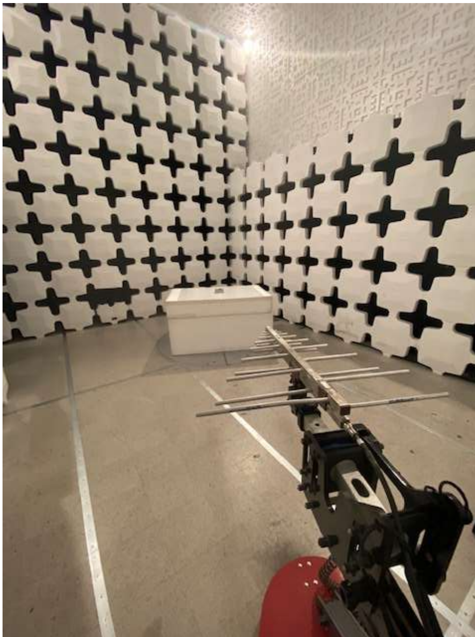
Figure 7. Radiated Emissions Test Configuration (200 MHz to 1 GHz), Internal Antenna
