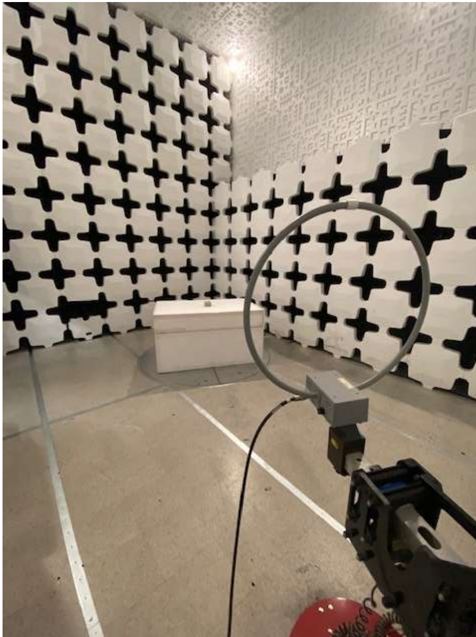
Figure 3. Radiated Emissions Test Configuration below 30 MHz, Internal Antenna
