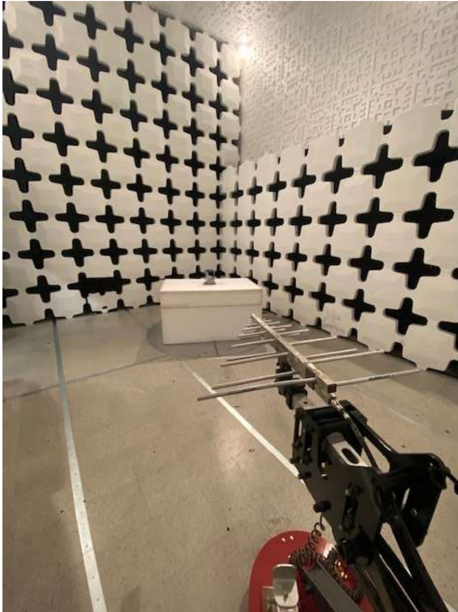
Figure 8. Radiated Emissions Test Configuration (200 MHz to 1 GHz), External Antenna
