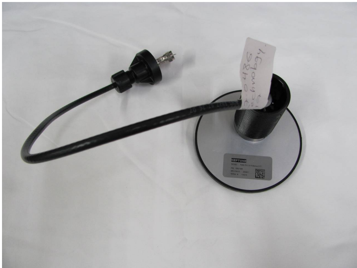
Figure 4. Standard Gain Pit Antenna, Bottom
