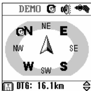
Compass Screen – Guides where to go for the destination. Upward direction is your heading direction.
