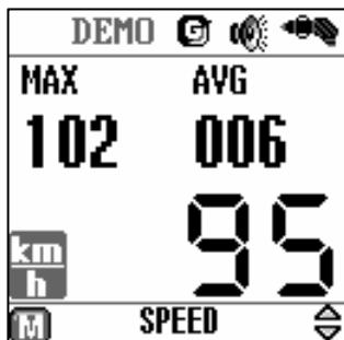
Speed Screen – Displays current speed, maximum speed and average speed.
