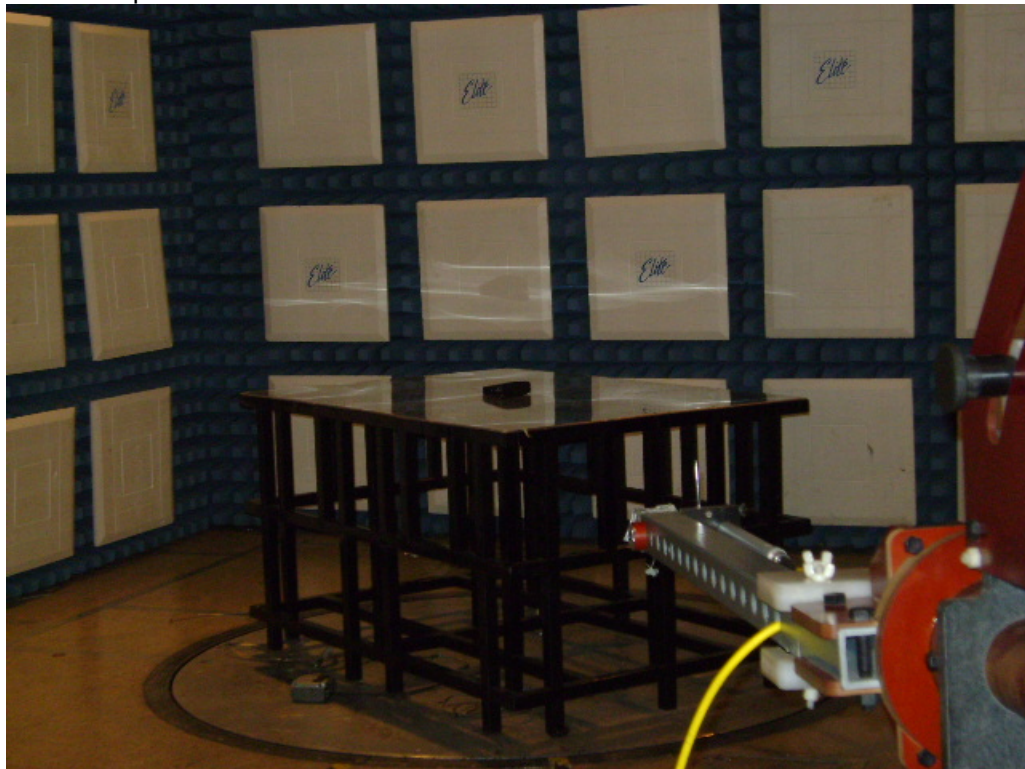
Test Setup for Radiated Emissions – 908MHz – Vertical Polarization - Transmitter
