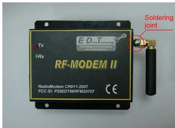
Before soldering antenna screw surface is opened by 45-degree cutting as shown below
