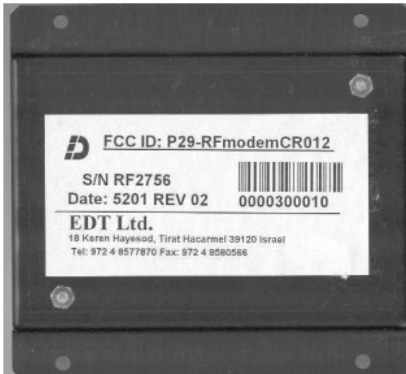
Figure 2: The identification label is attached to the back panel of the RF modem
