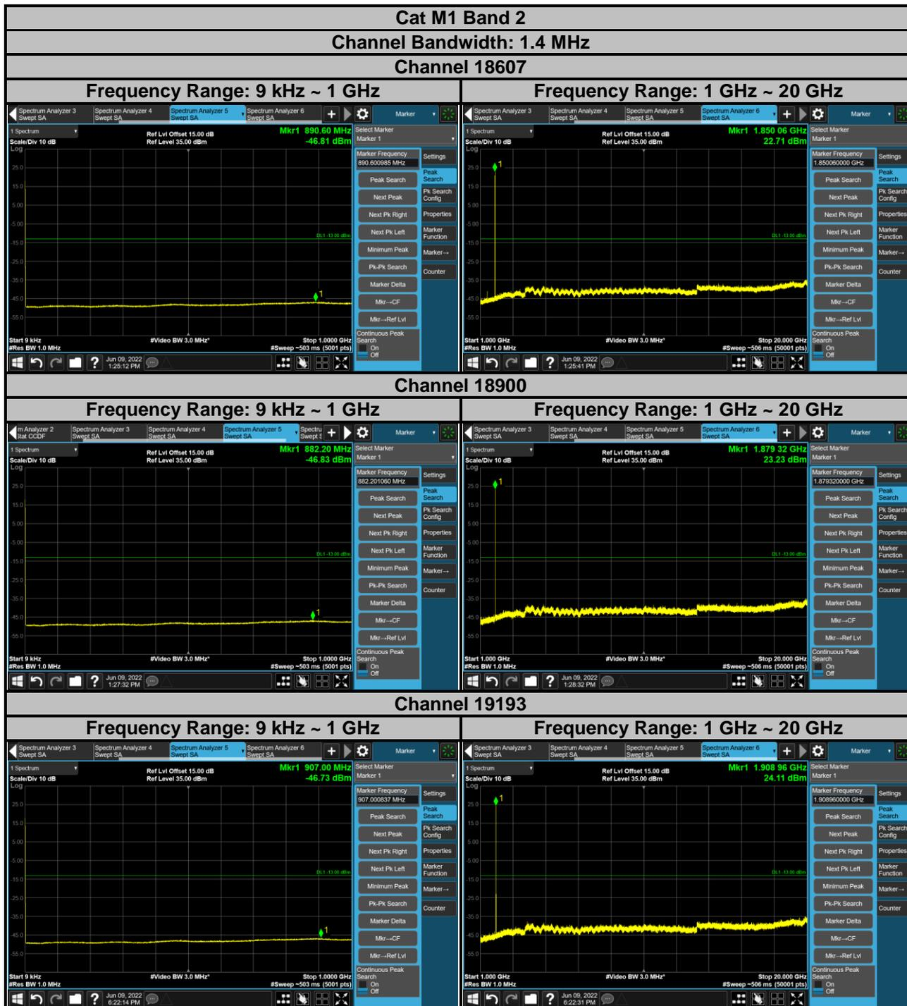
Note: The signal over the limit in 9 kHz is from spectrum analyzer.
