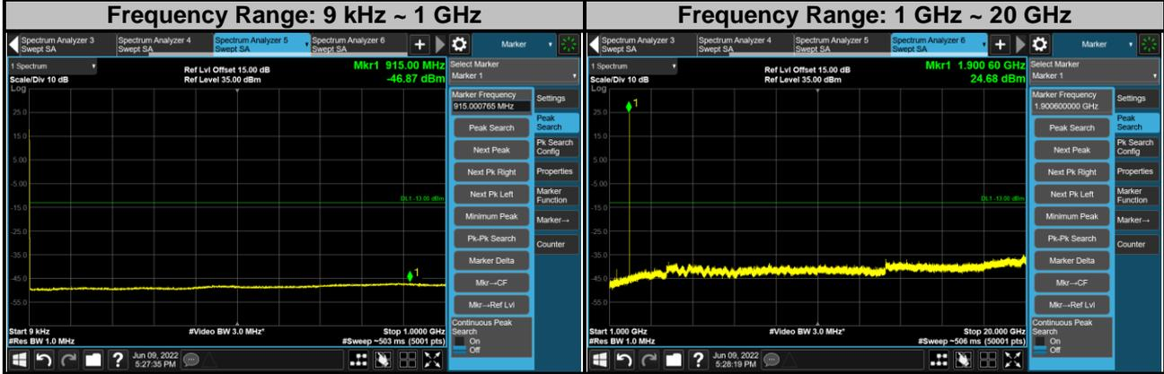
Note: The signal over the limit in 9 kHz is from spectrum analyzer.
