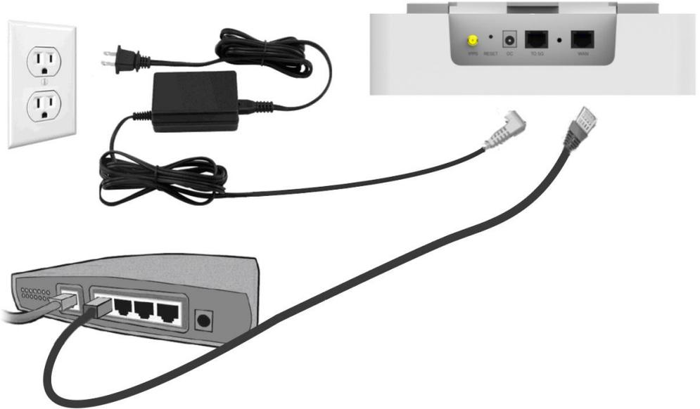
1. Small cell device provides mobile network SON ( Self-Organizing Network ) , it is plug& play which can auto configuration to install.
