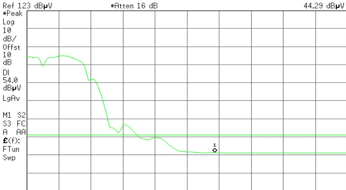
Start 2.460 00 GHz #Res BW 1 MHz #VBW 10 Hz Stop 2.500 00 GHz Sweep 3.119 s (601 pts)
