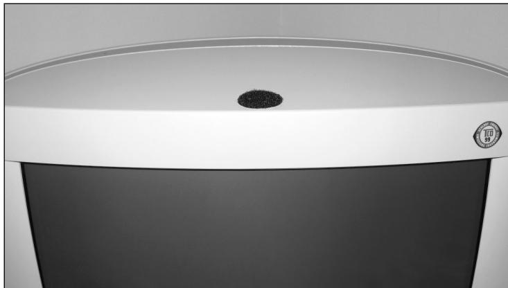
Figure 2-3. Velcro Pad Attached to a Monitor
