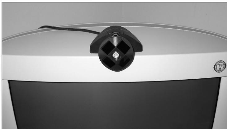
Figure 2-4. Monitor Sensor Attached to the Velcro Pad
