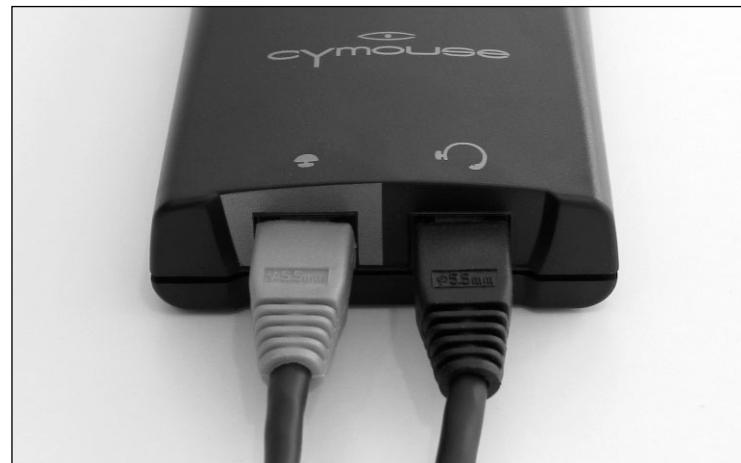
Figure 2-2. Connecting the Monitor Sensor Cable
