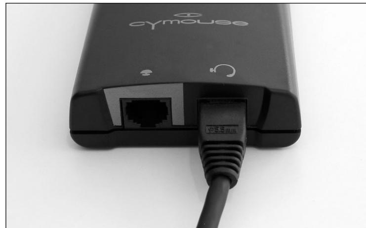
Figure 2-1. Connecting the Cymouse Headset Cable
