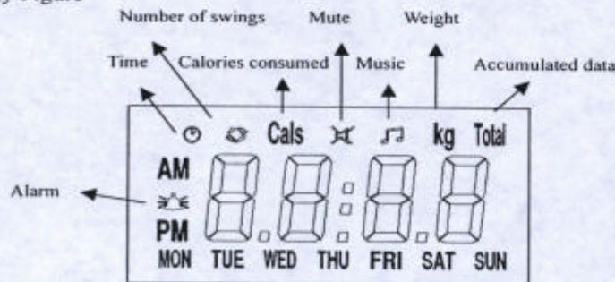
**1.Total / Alarm switch :** To switch OFF the alarm, stop alarm and music playing. Check the accumulated time, calories consumption and total number of swings that day.
